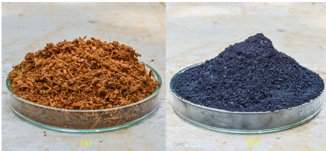
Fig. 3. Basin materials (a) coco peat (b) powdered charcoal.
