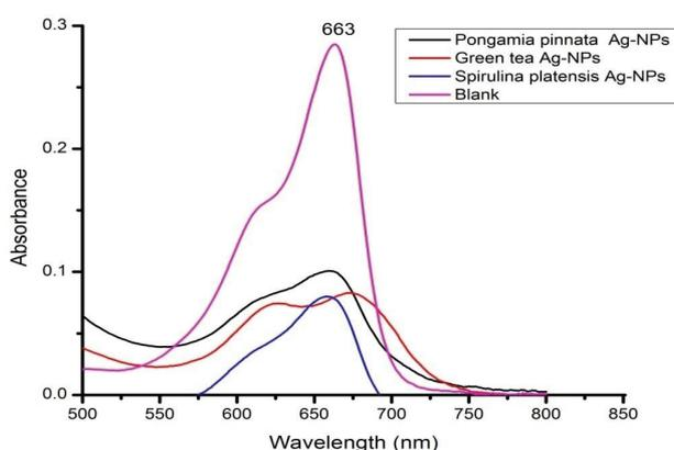
Fig. 6. a. UV VIS Spectra for MB and MB with Ag-NPs after 120 min.
