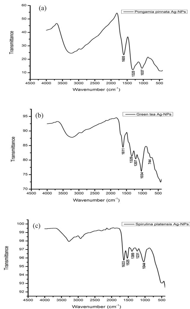
Fig. 4. FTIR analysis for (a) *Pongamia pinnata* Ag-NPs (b) Green tea Ag-NPs (c) *Spirulina platensis* Ag-NPs.
