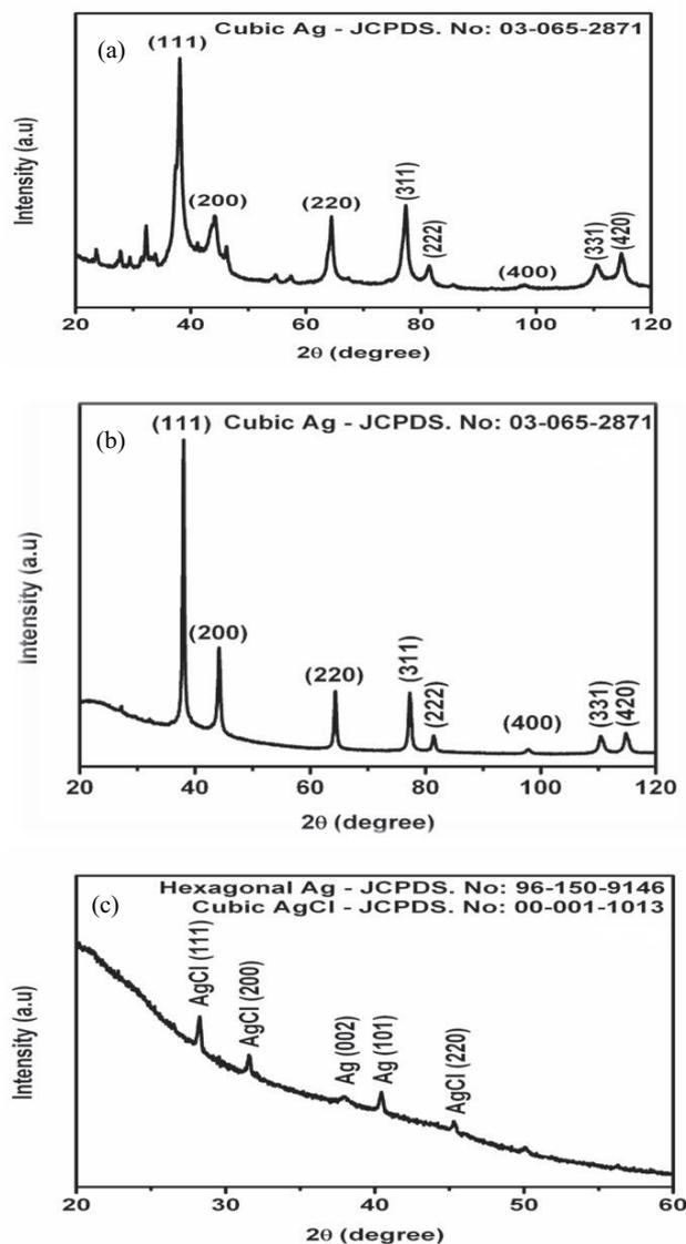
Fig. 3. XRD analysis for (a) *Pongamia pinnata* Ag-NPs (b) Green tea Ag-NPs (c) *Spirulina platensis* Ag-NPs.
