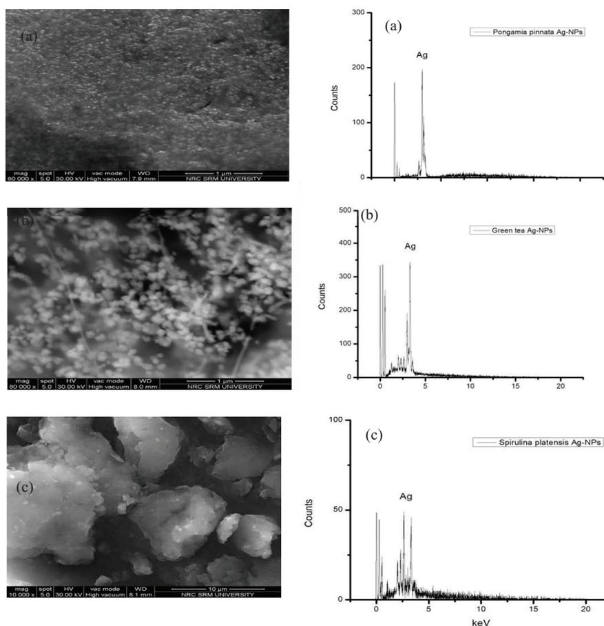
Fig. 5. SEM and EDX analysis for (a) *Pongamia pinnata* Ag-NPs (b) Green tea Ag-NPs (c) *Spirulina platensis* Ag-NPs.
