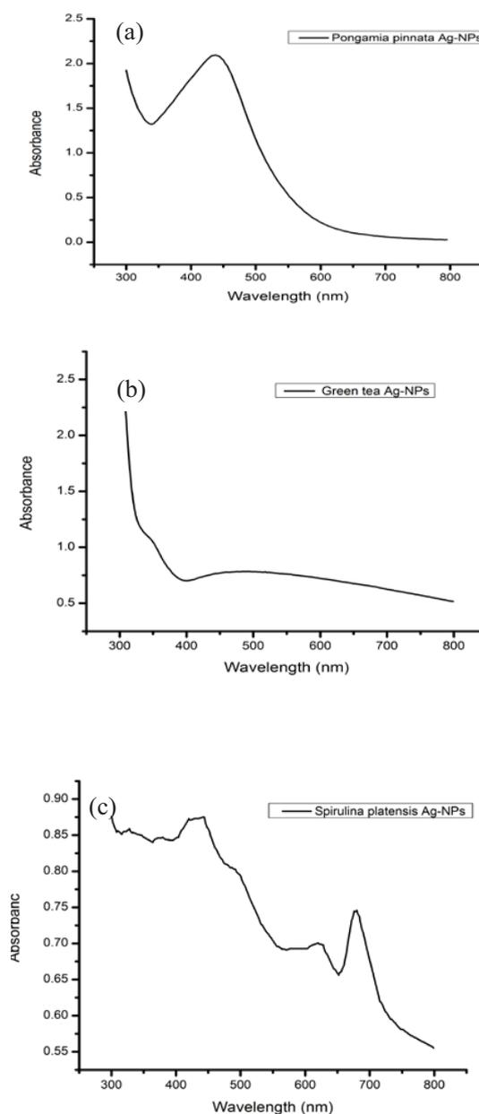
Fig. 2. UV VIS Spectroscopy for (a) *Pongamia pinnata* Ag-NPs (b) Green tea Ag-NPs (c) *Spirulina platensis* Ag-NPs.
