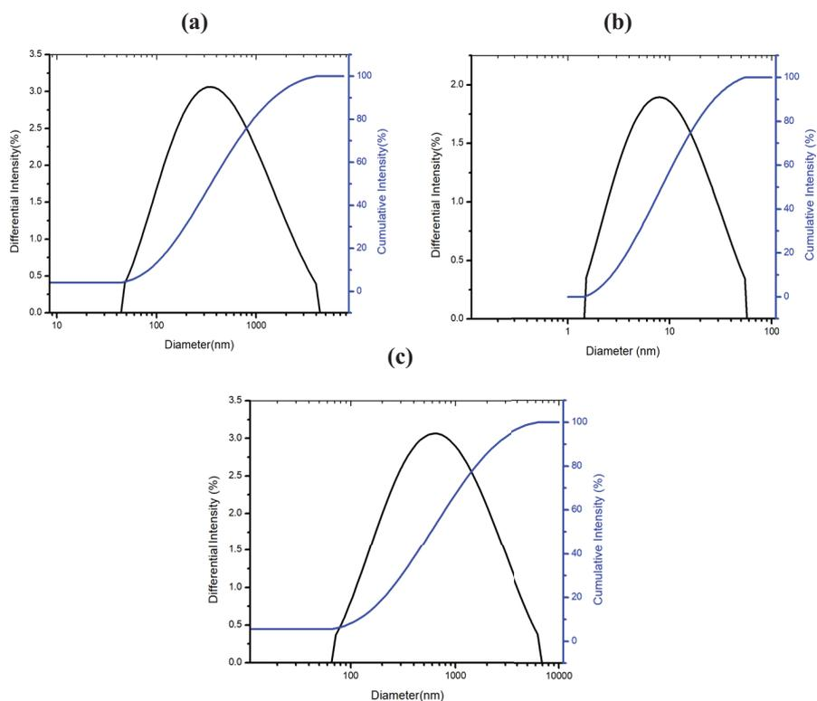
Fig. S2. Particle size analysis for (a) *Pongamia Pinnata* Ag-NPs (b) Green tea Ag-NPs (c) *Spirulina Platensis* Ag-NPs.
