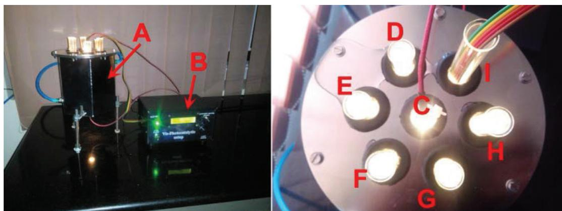
Fig. 1. Photographic images of developed visible photo-catalytic setup, (A) Water cooled chamber, (B) PID Intensity controller, (C) 1000 W tungsten-halogen lamp, (D–H) test tube having sample and dye, (I) test tube having BH1750 intensity sensor.
