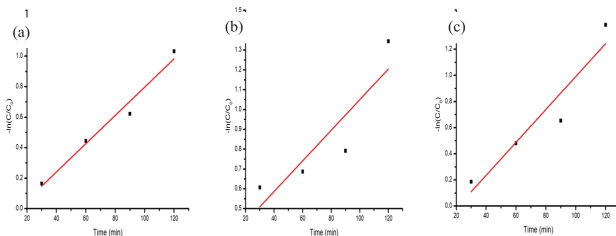
Fig. 6. c. First-order kinetics plots for MB using (a) *Pongamia pinnata* Ag-NPs (b) Green tea Ag-NPs (c) *Spirulina platensis* Ag-NPs after 120 min.
