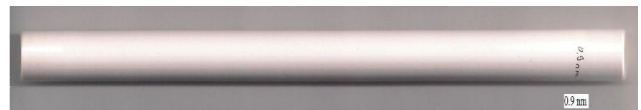
Fig. 3a. Virgin ceramic titanium dioxide NF membrane with pore size of 0.9 nm, length = 19 cm, ID = 7 mm, OD = 10 mm.
