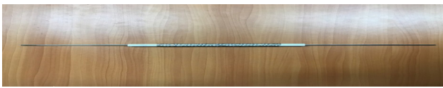
Fig. 3d. Represents ceramic membrane as shown in Fig. 3a and the outside electrode as shown in Fig. 3b was warped around the outer wall of tubular ceramic membrane.
