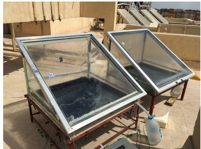
Fig. 1. Front view of the two solar stills.
