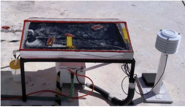
Fig. 3. Experimental setup of double slope solar still.
