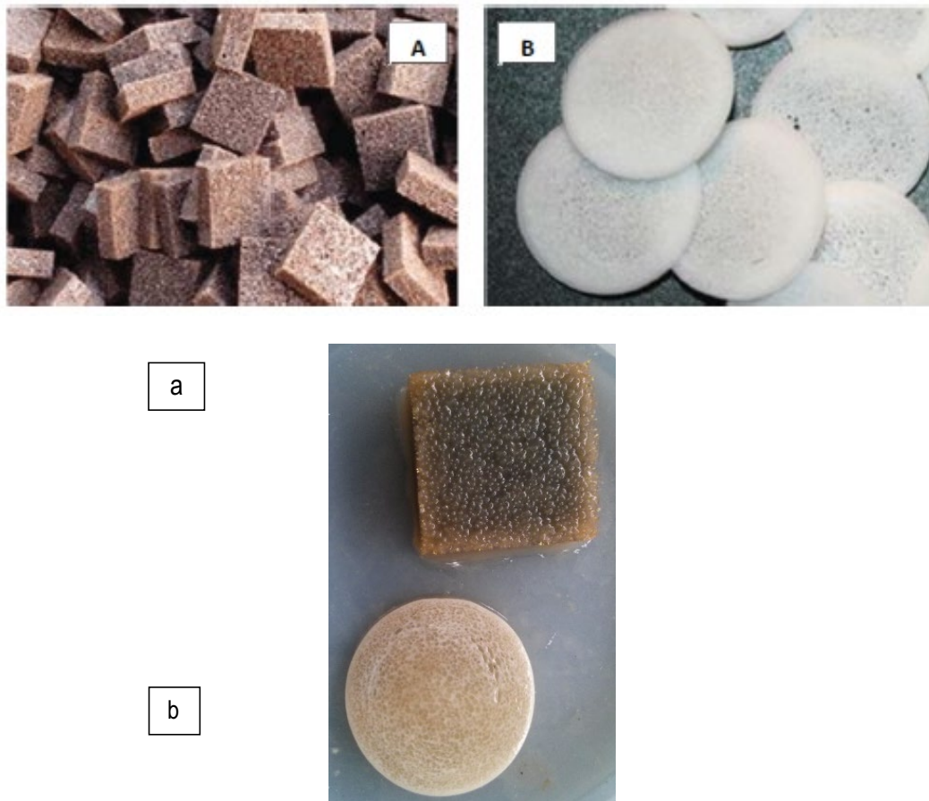
Fig. 2. Biomass carriers embedded in the MBR post-treatment. (a) Levapor biocarrier and (b) Mutag Biochip.
