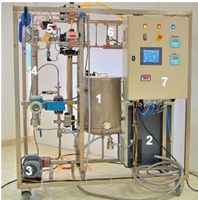
Fig. 2. Presentation of the nanofiltration pilot used in this study: (1) feed tank; (2) temperature control loop; (3) pressure pump; (4) 2.5" stainless steel pressure vessel; (5) pressure regulating valve; (6) sampling loop; (7) programmable logic controller.
