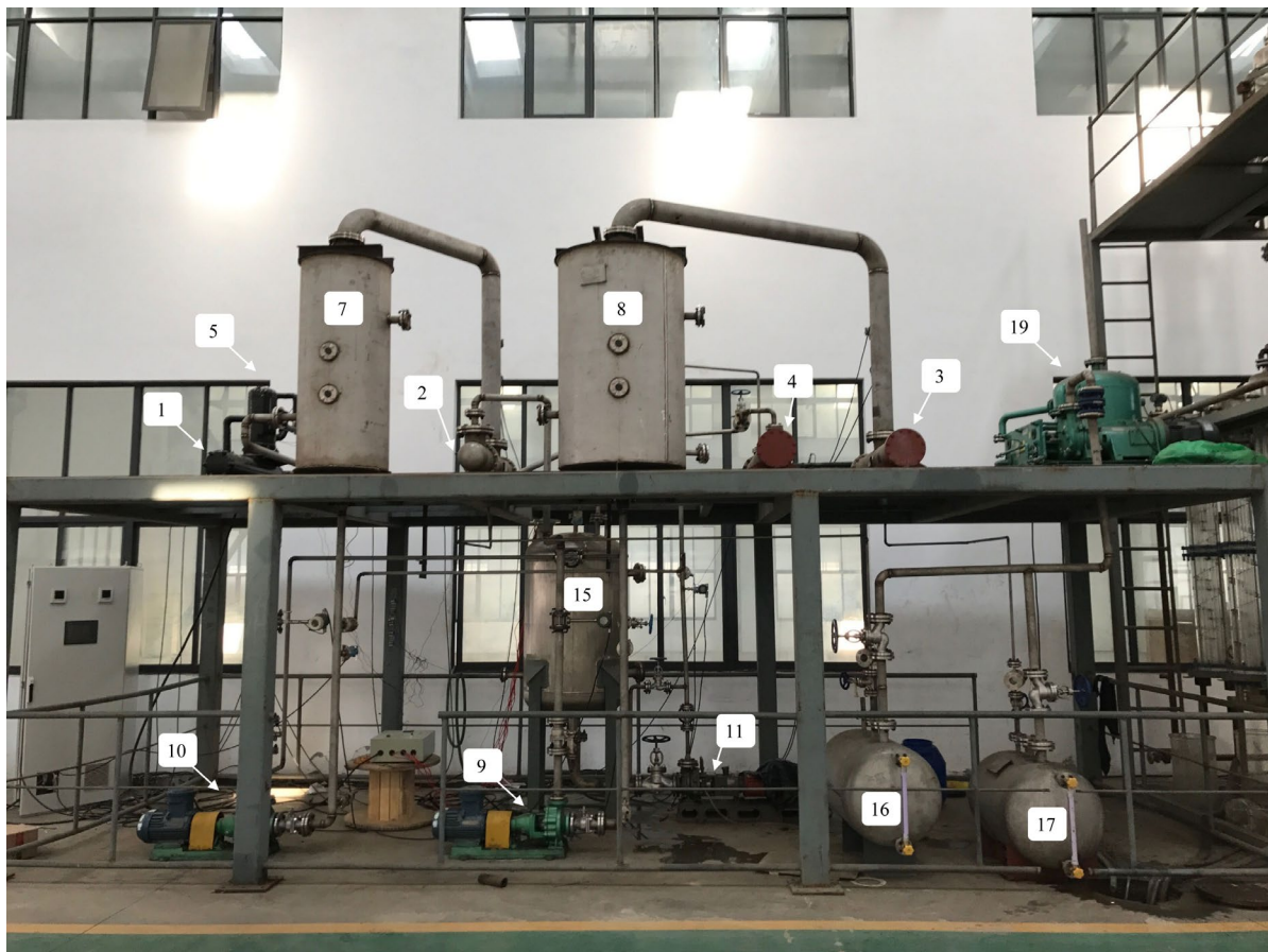
Fig. 9. Experimental device of the double-effect indirect heat pump distillation system.
