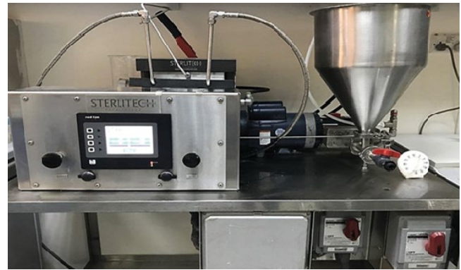
Fig. 1. Lab-scale membrane testing skid (Sterlitech Corporation, USA).
