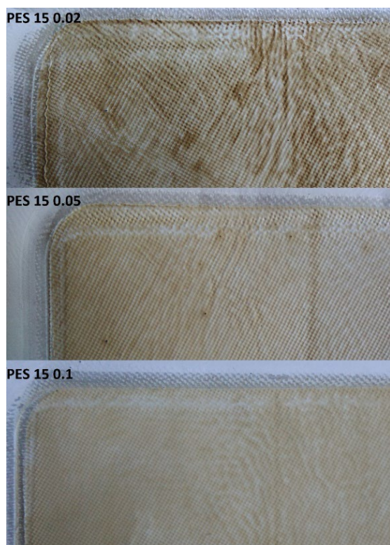
Fig. 7. Photographs of membrane surfaces after filtration: PES 15 0.02, PES 15 0.05, and PES 15 0.1.
