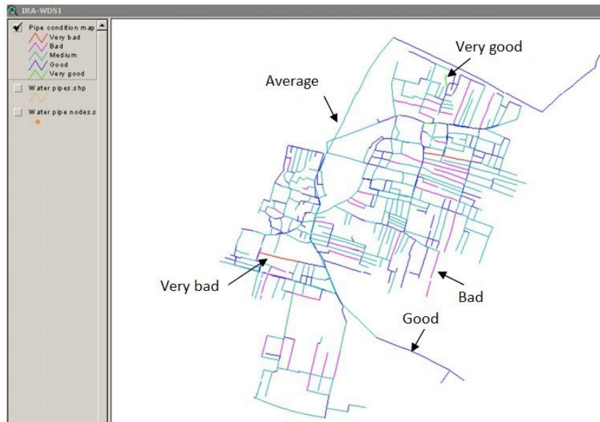
Fig. 2. Illustration of the possibilities of the IRA-WDS model (software and manual for risk assessment of contrast intrusion into water distribution systems)-to determine the level of risk of failure in a water supply network [22].
