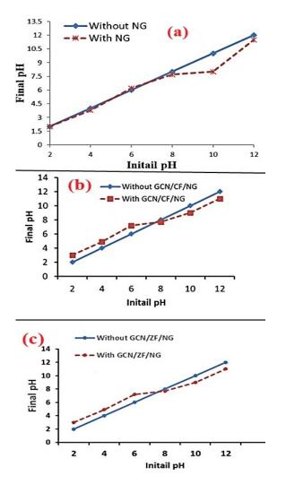
Fig. S3. pH of zero-point charge for (a) NG, (b) GCN/CoFe $_2O_4/$  NG, and (c) GCN/ZnFe $_2O_4/NG$  photocatalysts.
