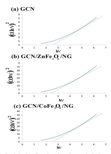
Fig. 8. Resultant Tauc plots of  $(\alpha\eta\nu)^2$  vs.  $\eta\nu$  for bandgap determination of (a) GCN, (b) GCN/ZnFe<sub>2</sub>O<sub>4</sub>/NG, and (c) GCN/CoFe<sub>2</sub>O<sub>4</sub>/NG.
