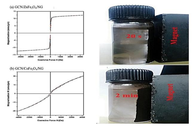
Fig. 10. Hysteresis curves of the (a) GCN/ZnFe<sub>2</sub>O<sub>4</sub>/NG and (b) GCN/CoFe<sub>2</sub>O<sub>4</sub>/NG heterojunctions and quick magnetic separation.
