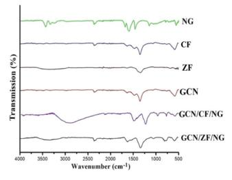
Fig. S1. FTIR spectra of NG,  $ZnFe_2O_4$ ,  $CoFe_2O_4$ , GCN, GCN/ CoFe<sub>2</sub>O<sub>4</sub>/NG, and GCN/ZnFe<sub>2</sub>O<sub>4</sub>/NG photocatalysts.
