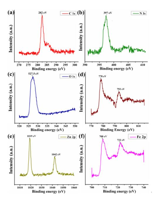
Fig. 7. XPS spectra of GCN/CoFe<sub>2</sub>O<sub>4</sub>/NG and GCN/ZnFe<sub>2</sub>O<sub>4</sub>/NG heterojunctions. Spectra of (a) C 1s, (b) N 1s, (c) O 1s, (d) Co 2p<sup>3</sup>, (e) Zn 2p<sup>3</sup>, and (f) Fe 2p<sup>3</sup>.
