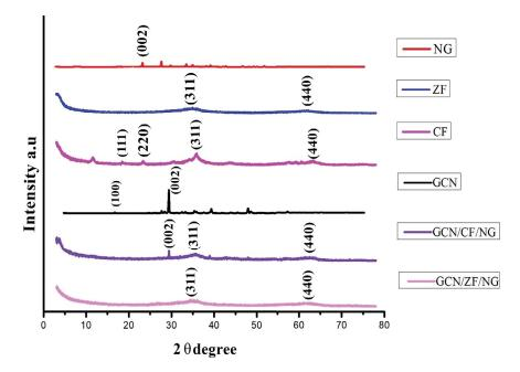
Fig. 5. XRD patterns of NG, ZnFe<sub>2</sub>O<sub>4</sub>, CoFe<sub>2</sub>O<sub>4</sub>, GCN, GCN/CoFe<sub>2</sub>O<sub>4</sub>/NG, and GCN/ZnFe<sub>2</sub>O<sub>4</sub>/NG composites.
