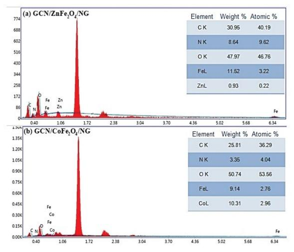
Fig. 6. EDS spectra of (a) GCN/ZnFe<sub>2</sub>O<sub>4</sub>/NG and (b) GCN/CoFe<sub>2</sub>O<sub>4</sub>/NG heterojunctions.
