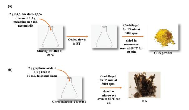
Fig. 1. Schematic illustration of (a) GCN and (b) NG synthesis using hydrothermal method.
