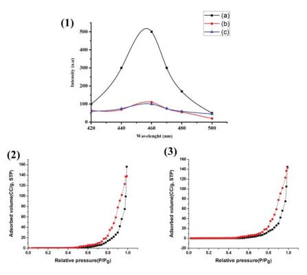
Fig. 9. (1) PL spectra of (a) GCN, (b) GCN/CoFe<sub>2</sub>O<sub>4</sub>/NG, and (c) GCN/ZnFe<sub>2</sub>O<sub>4</sub>/NG. BET isotherm for (2) GCN/ZnFe<sub>2</sub>O<sub>4</sub>/NG and (3) GCN/CoFe<sub>2</sub>O<sub>4</sub>/NG heterojunctions.
