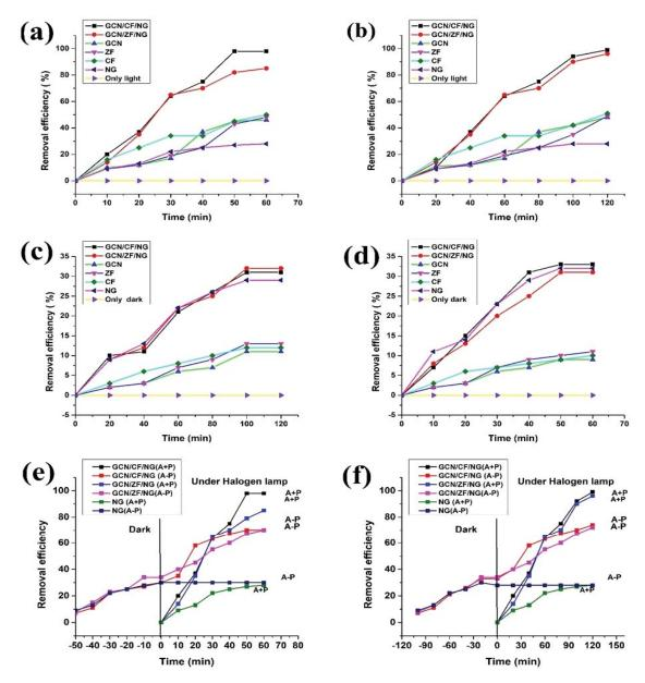
Fig. 11. Photocatalytic degradation of MO and MG over  $GCN/ZnFe_2O_4/NG$  and  $GCN/CoFe_2O_4/NG$  heterojunctions. Reaction conditions:  $[MO] = 1.5 \times 10^{-5}$  mol dm<sup>-3</sup>;  $[MG] = 1 \times 10^{-5}$  mol dm<sup>-3</sup>; [catalyst] = 50 mg/100 mL; pH = 4.0 (MO); 6 (MG); reaction time = 70 min (MG), and 140 min (MO).
