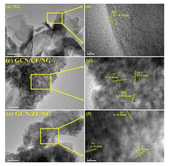
Fig. 3. TEM and HRTEM images of (a and b) pure NG, (c and d) GCN/CoFe<sub>2</sub>O<sub>4</sub>/NG, and (e and f) GCN/ZnFe<sub>2</sub>O<sub>4</sub>/NG photocatalysts.
