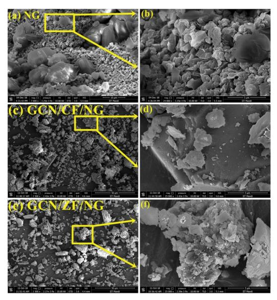
Fig. 4. SEM images of (a and b) pure NG, (c and d) GCN/CoFe<sub>2</sub>O<sub>4</sub>/NG, and (e and f) GCN/ZnFe<sub>2</sub>O<sub>4</sub>/NG photocatalysts.
