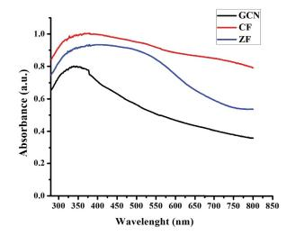
Fig. S2. UV-vis absorption spectra of  $\rm ZnFe_2O_{4'}$   $\rm CoFe_2O_{4'}$  and GCN.
