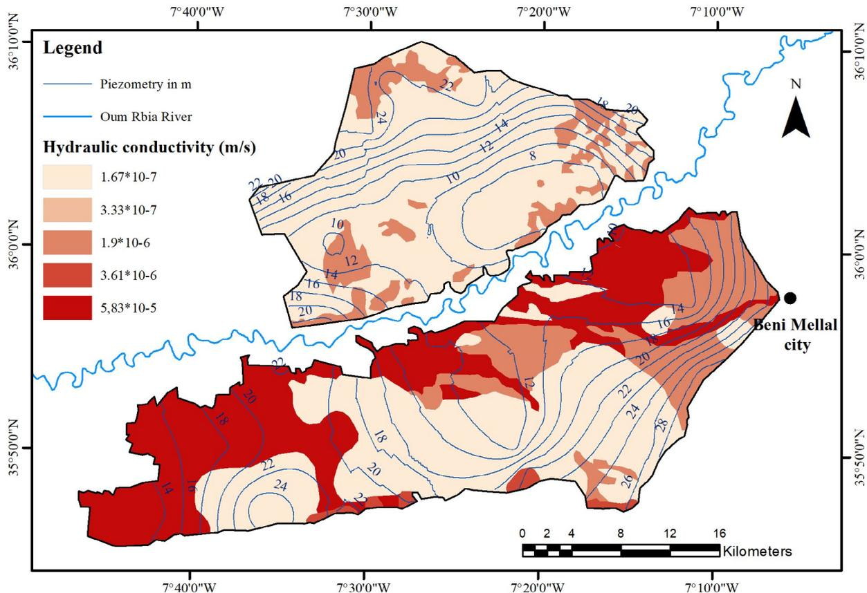
Fig. 7. Layering cards (piezometric maps and hydraulic conductivity).
