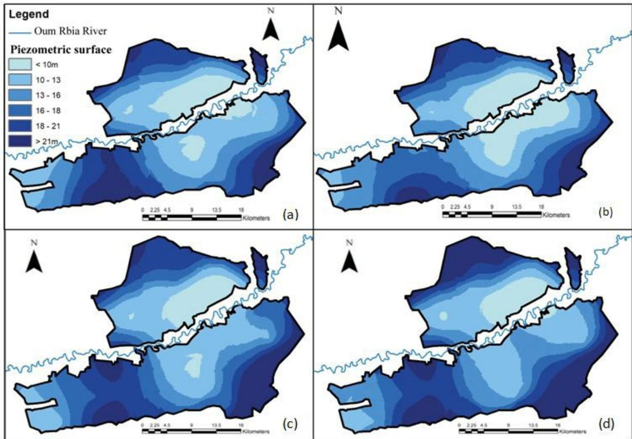
Fig. 3. Piezometric levels map (a) 2014, (b) 2015, (c) 2016, and (d) 2017, 200 mm × 140 mm (96 × 96 DPI).
