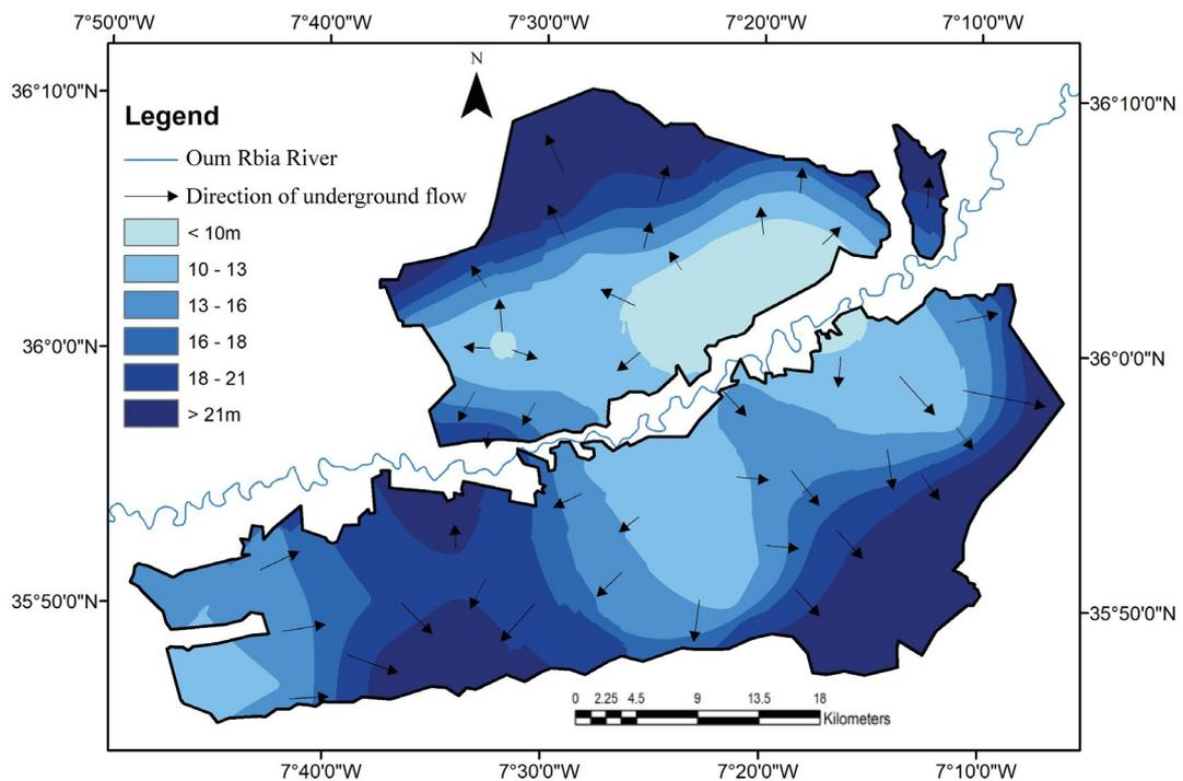
Fig. 4. Groundwater direction flow in the perimeter of Tadla.
