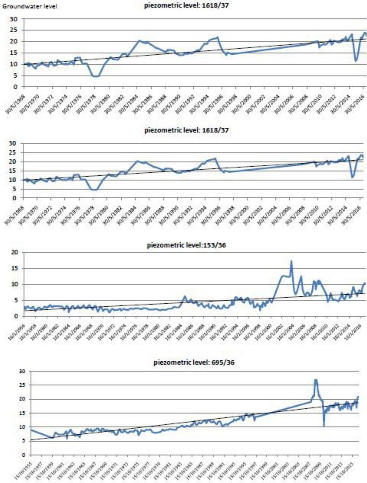
Fig. 6. Evolution of the piezometric levels at wells of Tadla perimeter, 130 × 169 mm (96 × 96 DPI).
