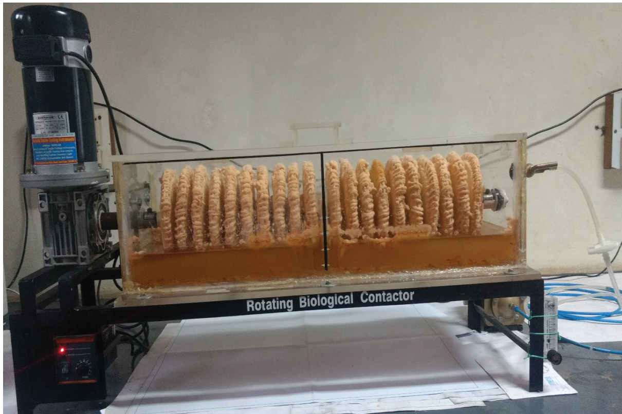
Fig. S7. Experimental setup of attached active live fungal biomass on PU covered discs in RBC reactor (before decolorization of CR dye wastewater).
