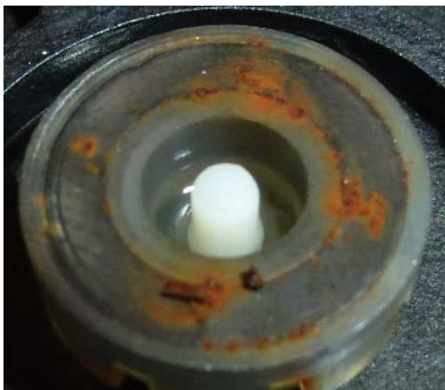
Fig. 9. View of the magnetic coupling of the water meter with iron deposits.
