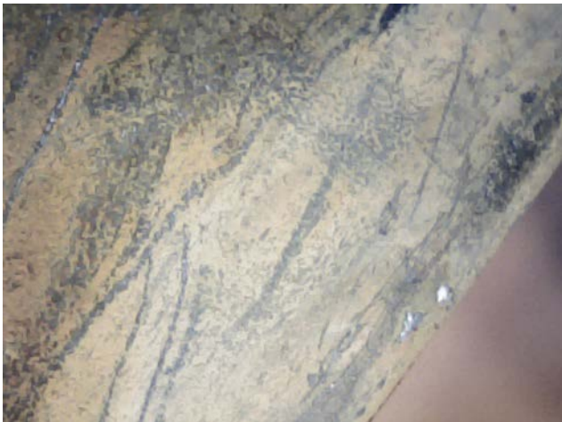
Fig. 6. Microscopic view (100x) of the rotor surface covered with calcium carbonate scaling.
