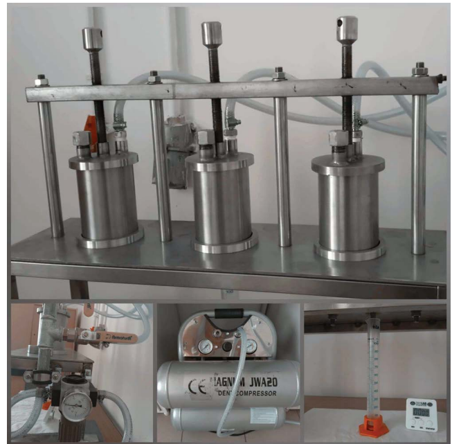
Fig. 1. Pressure filtration station.
