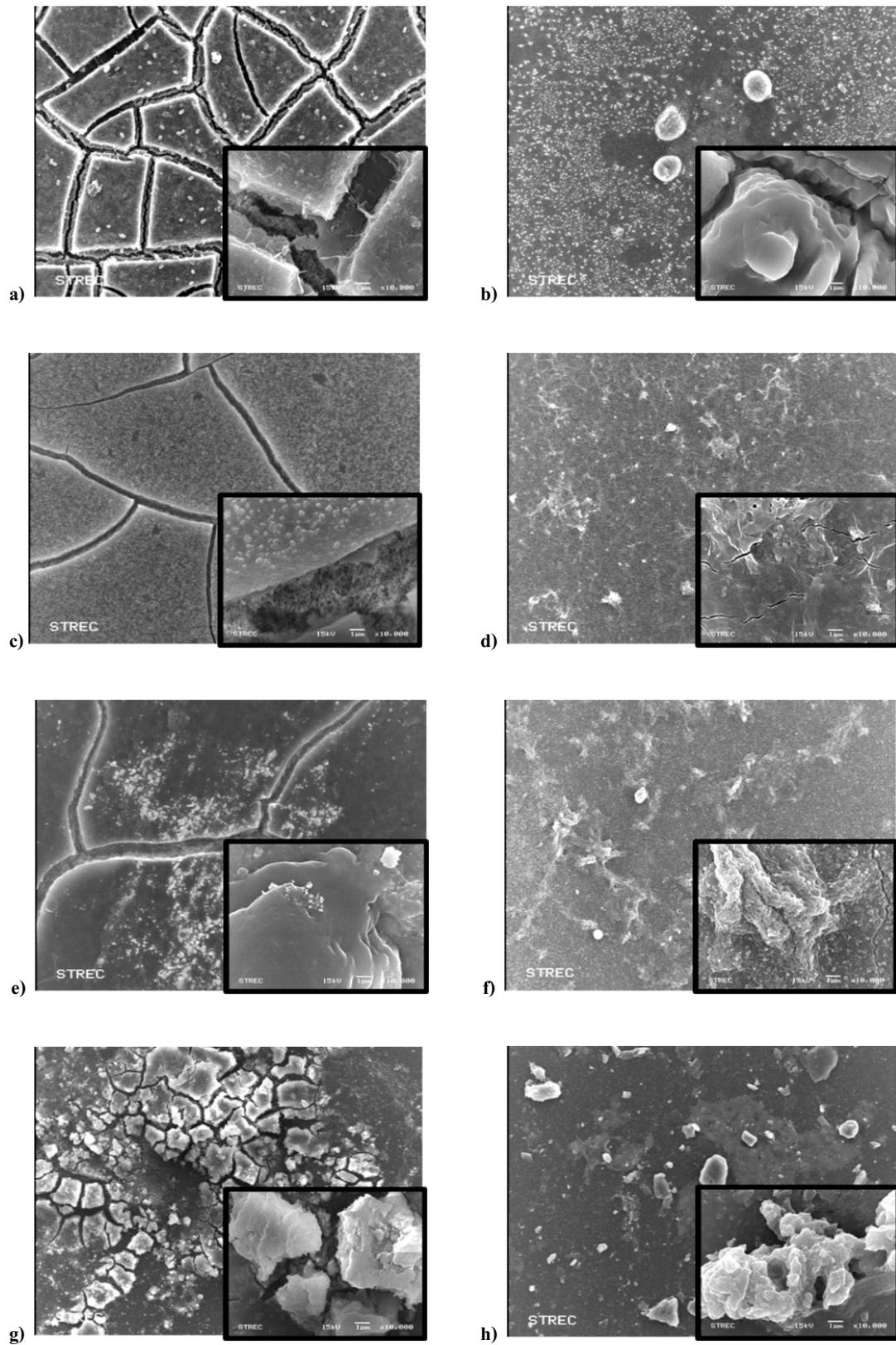
Fig. 5. SEM images of foulant on RO membranes (a) fouled membrane with  $\text{FeCl}_3$  coagulated leachate, (b) cleaned membrane ( $\text{FeCl}_3$  coagulated leachate), (c) fouled membrane fouled with 1.2  $\mu\text{m}$  filtrate, (d) cleaned membrane (1.2  $\mu\text{m}$  filtrate), (e) fouled membrane with 0.45  $\mu\text{m}$  filtrate, (f) cleaned membrane (0.45  $\mu\text{m}$  filtrate), (g) fouled membrane with 1 kDa filtrate, and (h) cleaned membrane (1 kDa filtrate).
