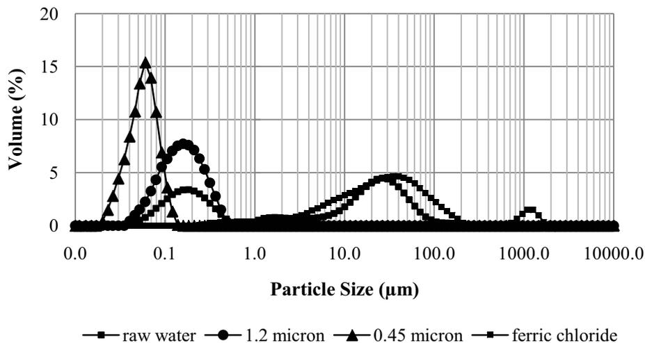
Fig. 1. Distribution of particle size in raw leachate, supernatant after  $\text{FeCl}_3$  coagulation, and filtrates through 1.2, 0.45 mm membranes.
