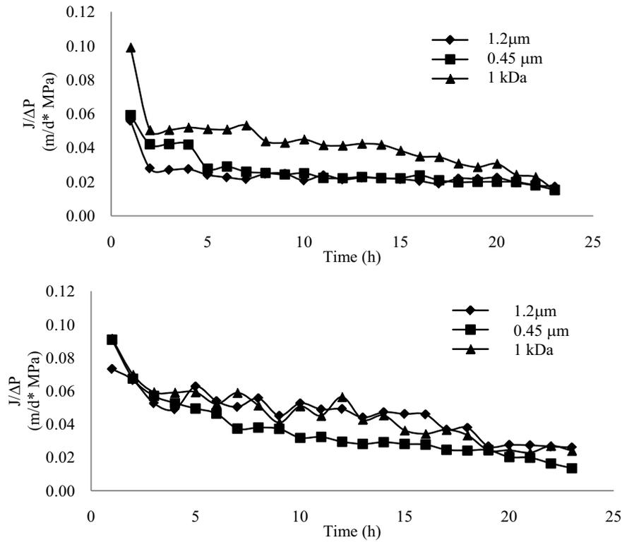
Fig. 2. Normalized flux with applied pressure for raw (upper) and FeCl<sub>3</sub> coagulated leachate (lower).
