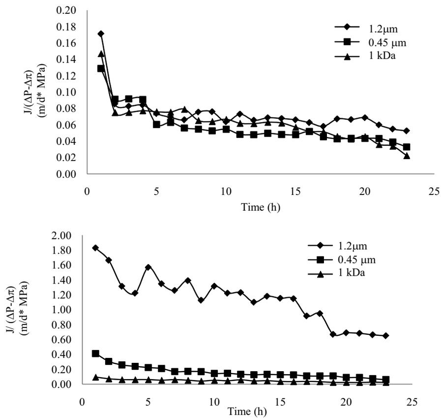
Fig. 3. Normalized flux with net pressure of raw (upper) and FeCl<sub>3</sub> coagulated leachate (lower).
