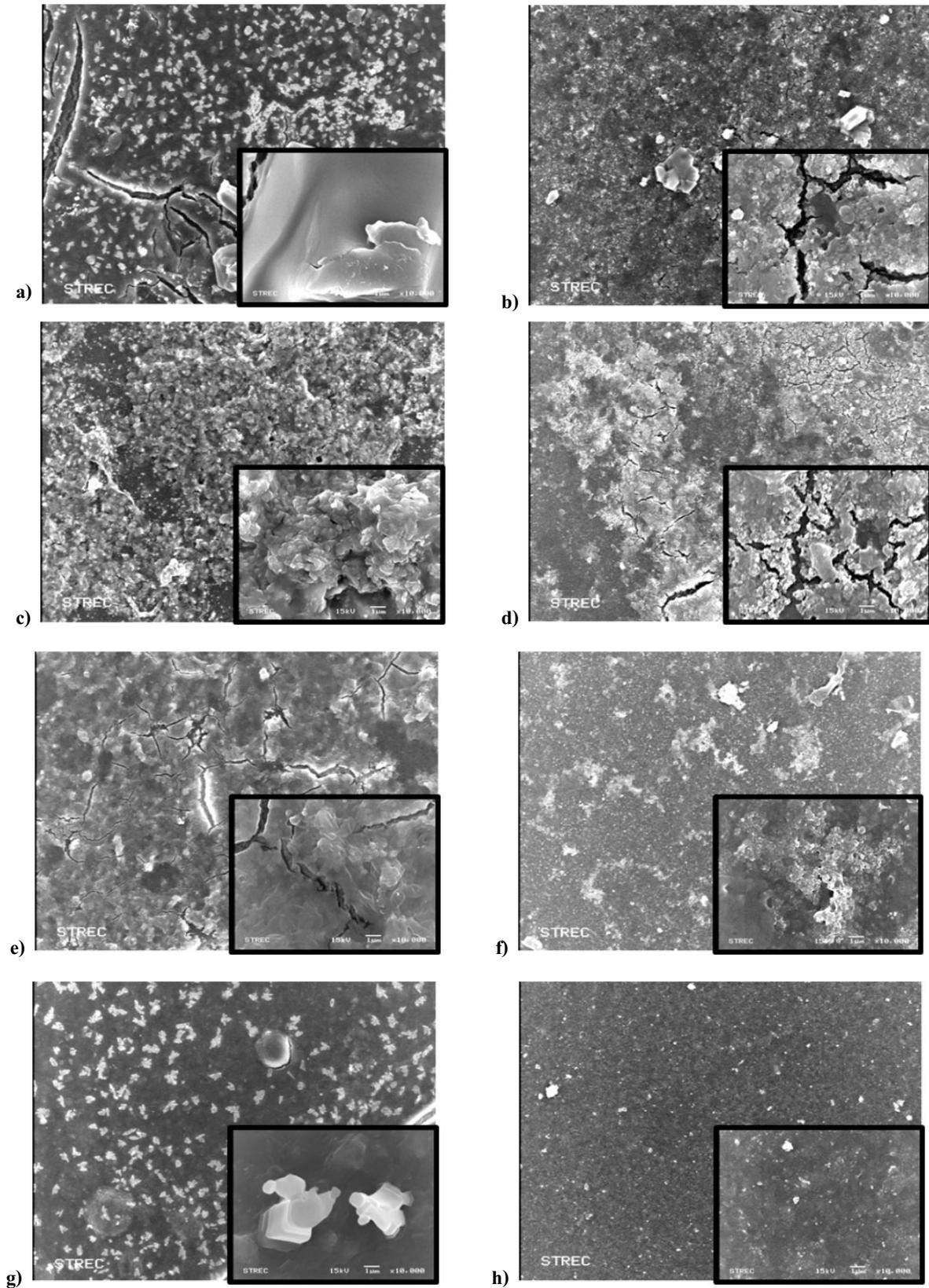
Fig. 4. SEM images of foulant on RO membranes (a) fouled membrane by raw leachate, (b) cleaned membrane (raw leachate), (c) fouled membrane by 1.2  $\mu\text{m}$  filtrate, (d) cleaned membrane (1.2  $\mu\text{m}$  filtrate), (e) fouled membrane with 0.45  $\mu\text{m}$  filtrate, (f) cleaned membrane (0.45  $\mu\text{m}$  filtrate), (g) fouled membrane with 1 kDa filtrate, and (h) cleaned membrane (1 kDa filtrate).
