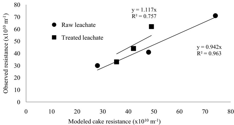
Fig. 6. Comparison of filtration resistance obtained from experiment and cake model.
