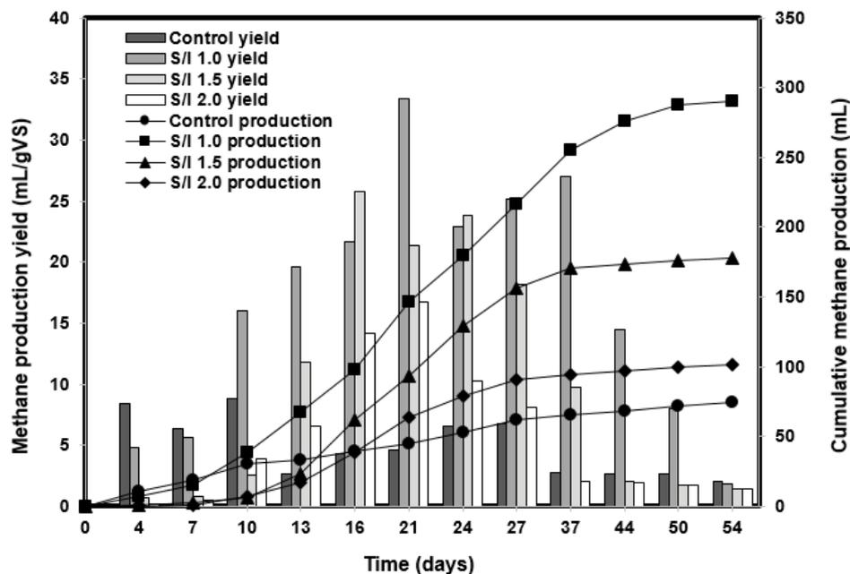
Fig. 8. Specific methane production yield and cumulative methane production at all S/I ratios.
