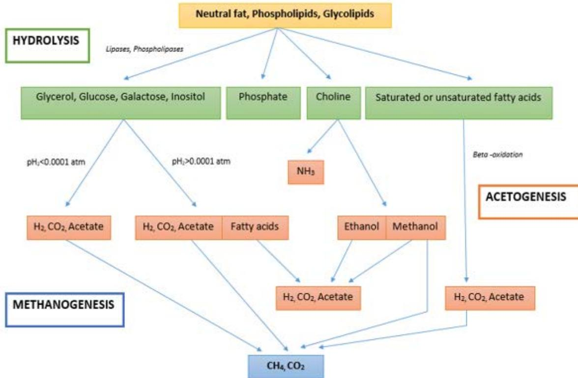
Fig. 1. Metabolic pathway of anaerobic degradation of fats [20].
