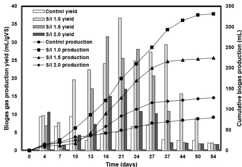
Fig. 7. Specific biogas production yield and cumulative biogas production at different S/I ratios.
