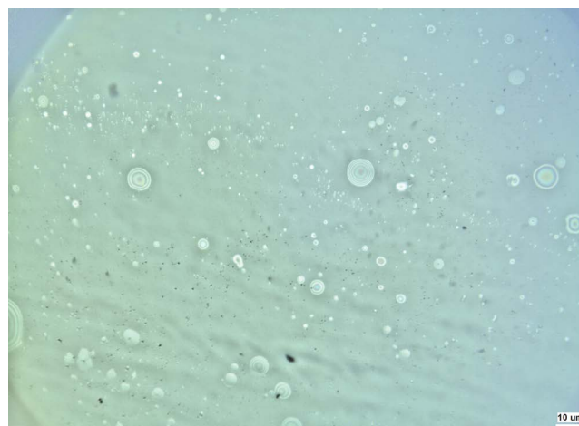
Fig. 5. Optical microscopy on the size of oil droplet.
