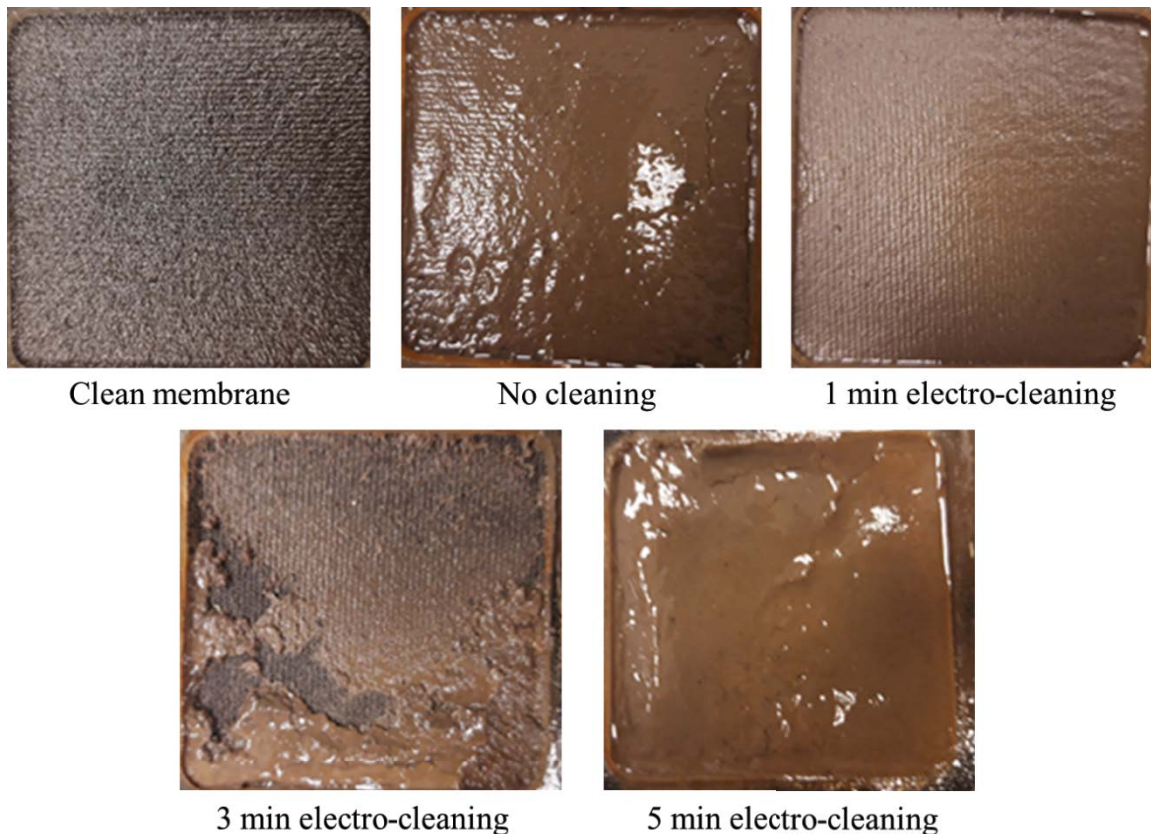
Fig. 10. The photos of the membranes before and after cleaning.
