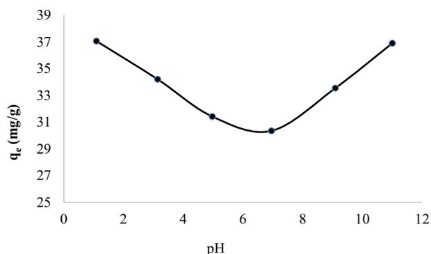
Fig. 4. Solution pH impact on methylene blue adsorption by  $\text{ZnCl}_2$  modified leaves powder of *Nitraria retusa* at room temperature.
