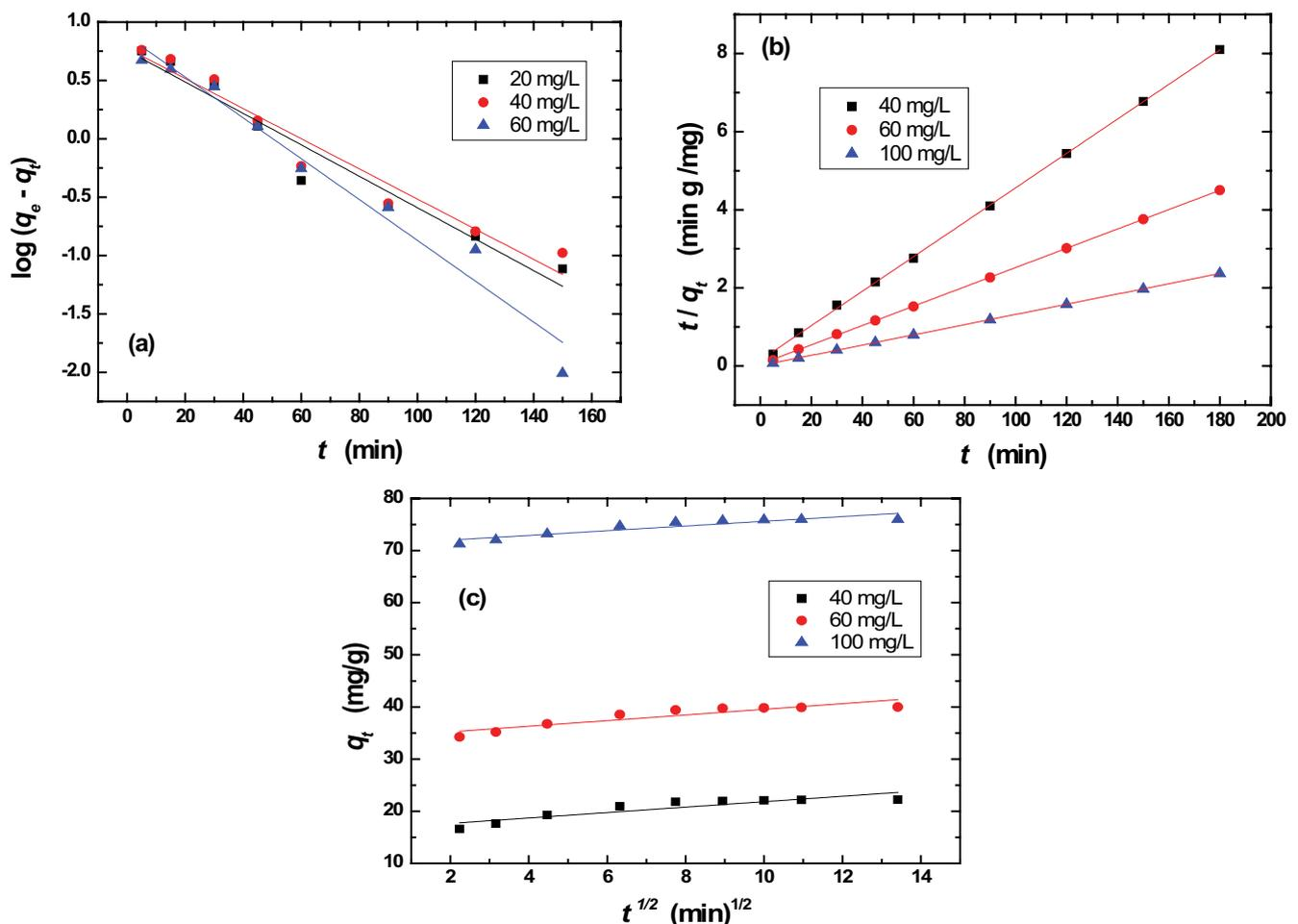
Fig. 7. (a) Pseudo-first-order, (b) Pseudo-second-order, and (c) diffusion of intra-particle kinetic models for methylene blue adsorption by ZnCl<sub>2</sub> modified leaves powder of *Nitraria retusa* at room temperature and solution pH of 6.
