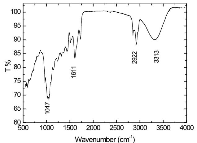
Fig. 3. Fourier-transform infrared spectroscopy for the ZnCl<sub>2</sub> modified leaves powder of *Nitraria retusa*.
