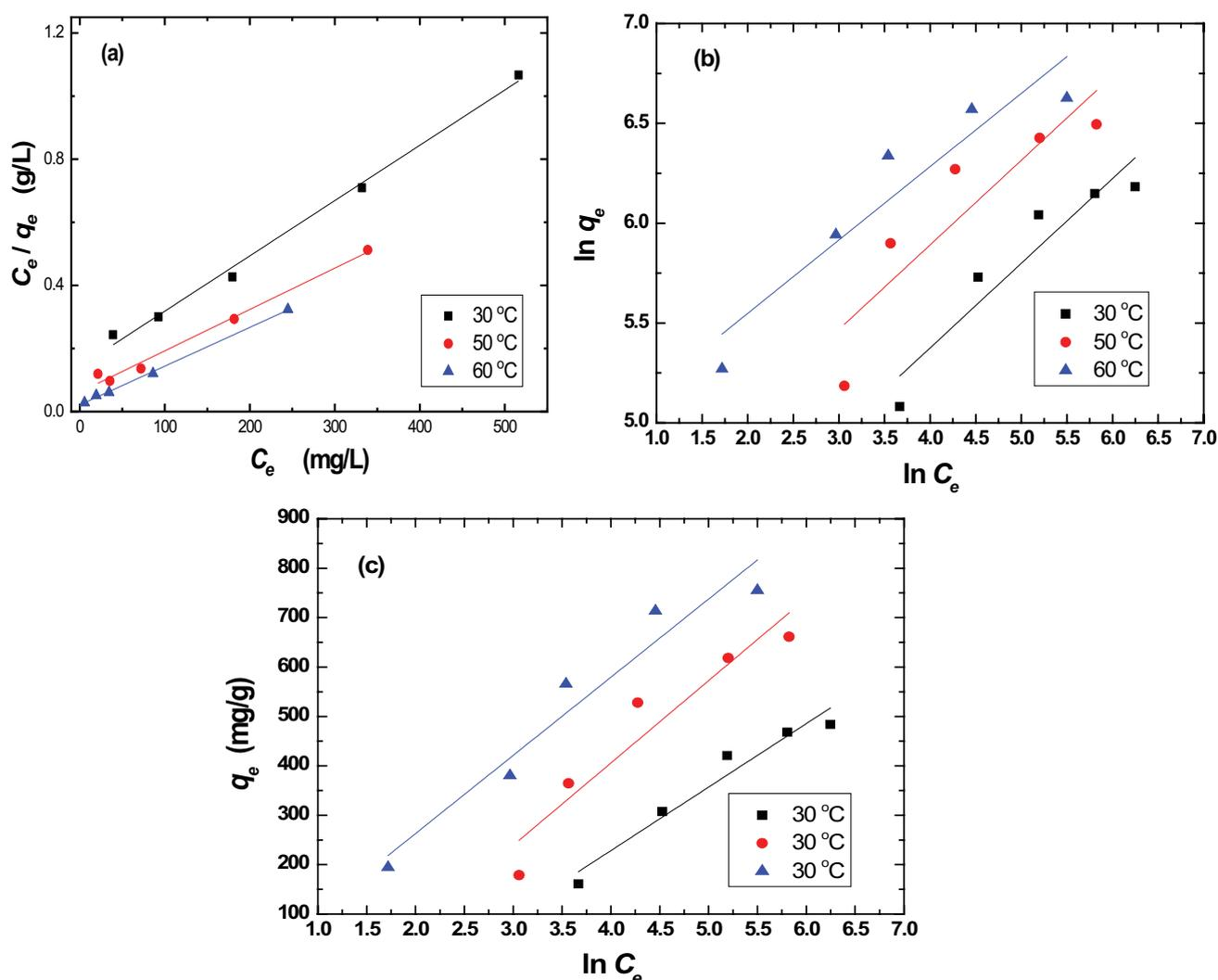
Fig. 8. (a) Langmuir, (b) Freundlich, and (c) Temkin isotherms for methylene blue adsorption by  $\text{ZnCl}_2$  modified leaves powder *Nitraria retusa* at three different temperature and solution pH of 6.
