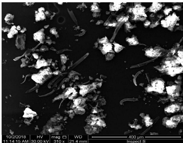
Fig. 1. Scanning electron microscopy for the ZnCl<sub>2</sub> modified leaves powder of *Nitraria retusa*.
