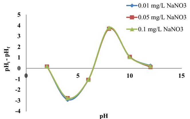
Fig. 2.  $\text{pH}_{\text{ZPC}}$  for the ZnCl<sub>2</sub> modified leaves powder of *Nitraria retusa*.
