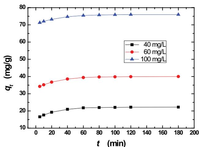
Fig. 6. Impact of the contact time on methylene blue adsorption by  $\text{ZnCl}_2$  modified leaves powder of *Nitraria retusa* at room temperature and solution pH of 6.
