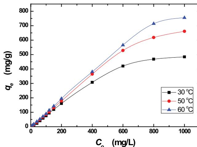
Fig. 5. Temperature and adsorbate initial concentration impacts on methylene blue adsorption by  $\text{ZnCl}_2$  modified leaves powder of *Nitraria retusa* at solution pH of 6.
