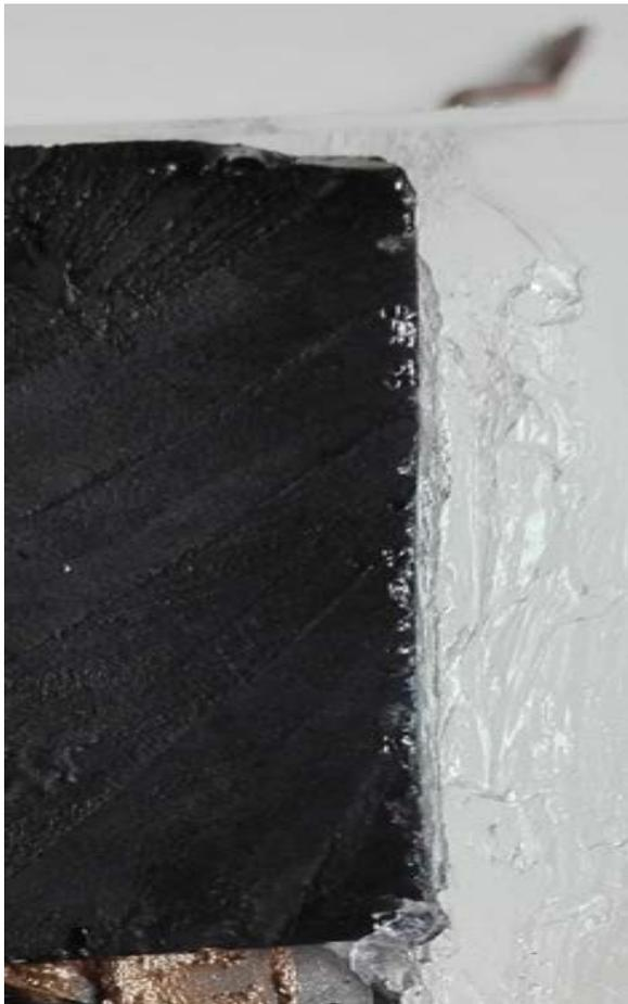
Fig. S1. Copper conductive adhesive and covered the bonding areas with silicone adhesive to prevent the oxidation of the copper adhesive by air.
