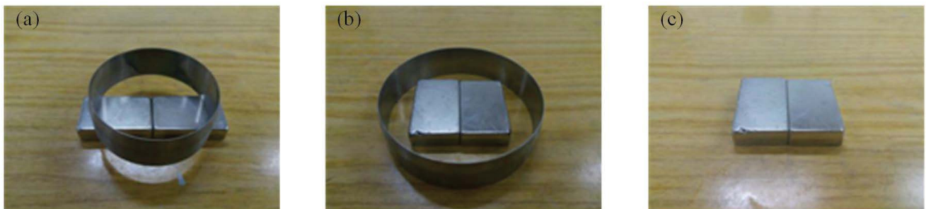
Fig. 2. Experimental setup of SMFs for the static treatment: (a) weak SMF (45 mT), (b) moderate SMF (150 mT), and (c) strong SMF (370 mT).
