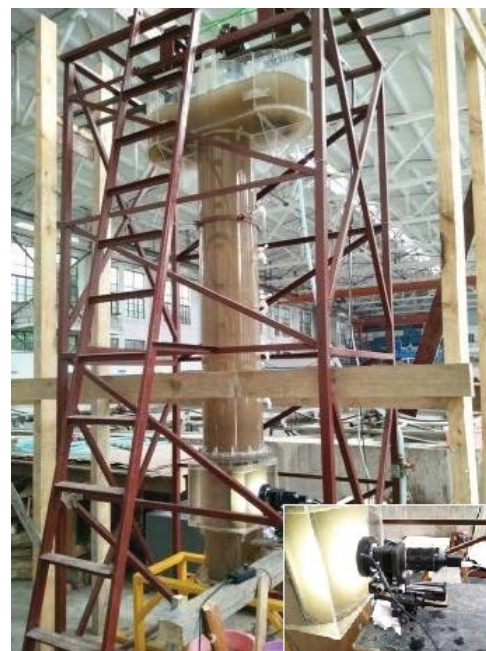
Fig. 2. Apparatus. (1) motor; (2) inlet; (3) grille; (4) grill connecting rod; (5) sampling port; (6) observation area; (7) camera; (8) personal computer.
