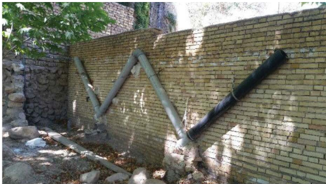
Fig. 4. Scheme of the used pipe pilot.
