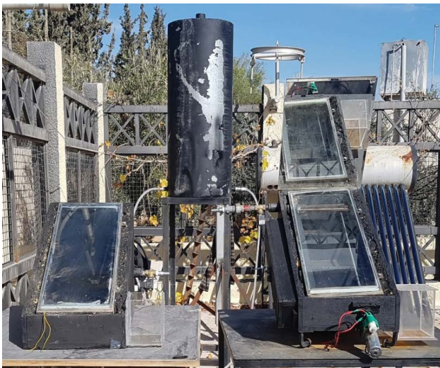
Fig. 10. Experimental setup of traditional and modified stills.
