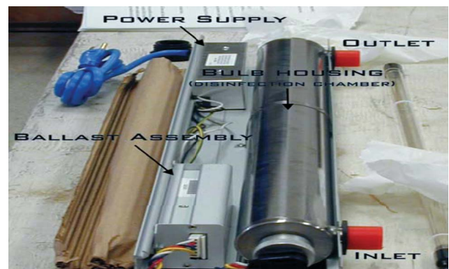
Fig. 1. Schematic of UV unit with cover removed [11].
