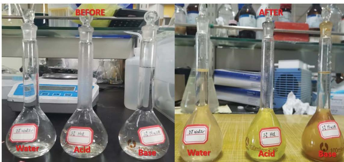
Fig. S1. Chemical solubility test experimental set-up (before and after the test).
