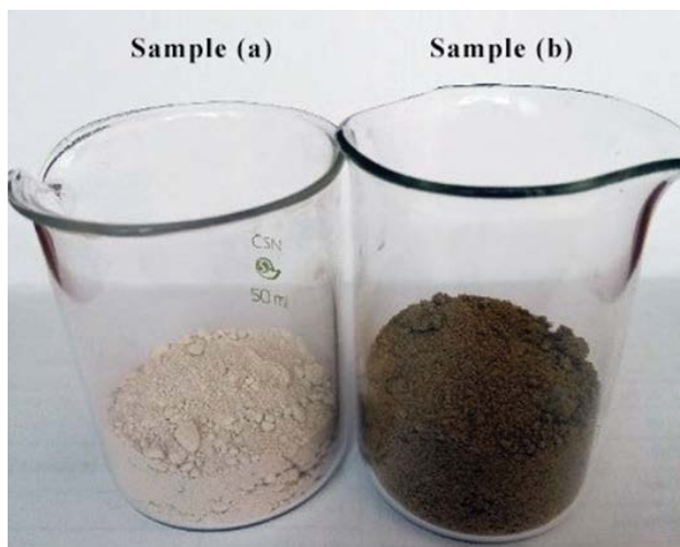
Fig. 4. Samples of natural (a) CaCO 3 (chalk) and (b) quartz-glaucinite sand taken from Zdolbuniv Quarry.
