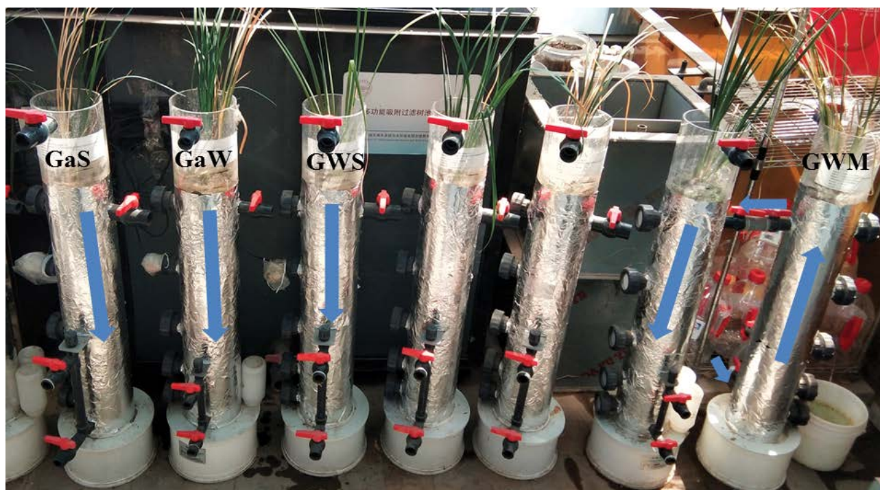
Fig. 1. Bioretention columns (GaS, GaW, GWS and GWM) in the greenhouse.
