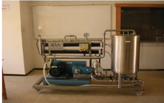
Fig. 1. Diagram and picture of the nanofiltration pilot plant. T: tank; P: feed pump; V: pressure regulation valves; M: NF/RO module; Pe: permeate recirculation; R: retentate recirculation; H: heat exchanger; 1: pressure sensor; 2: temperature sensor.
