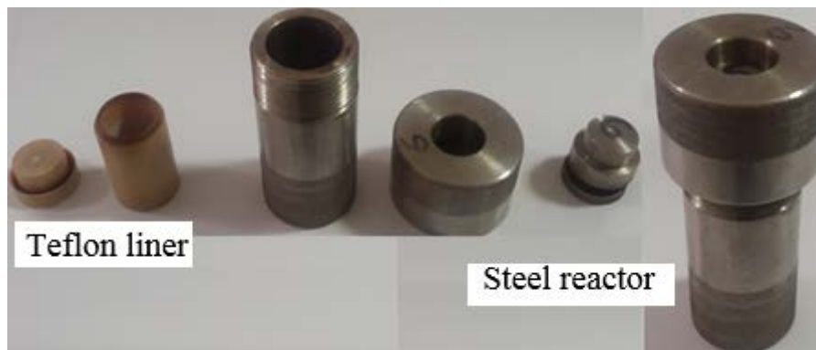
Fig. 2. Autoclave used in synthesis of nanoparticles.
