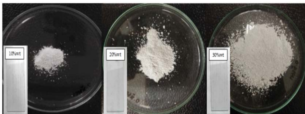
Fig. 3. CNT/TiO 2 with various ratios coating on a glass slide.
