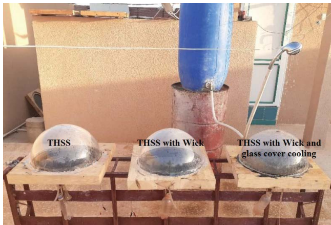
Fig. 2. Hemispherical solar still with a wick and glass cover cooling.
