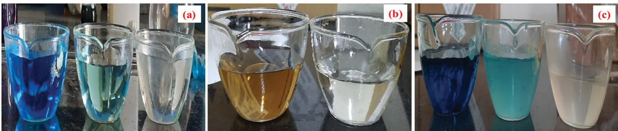
Fig. 9. Degradation of dye (a) methylene blue, (b) fast sulphon black, and (c) brilliant green.
