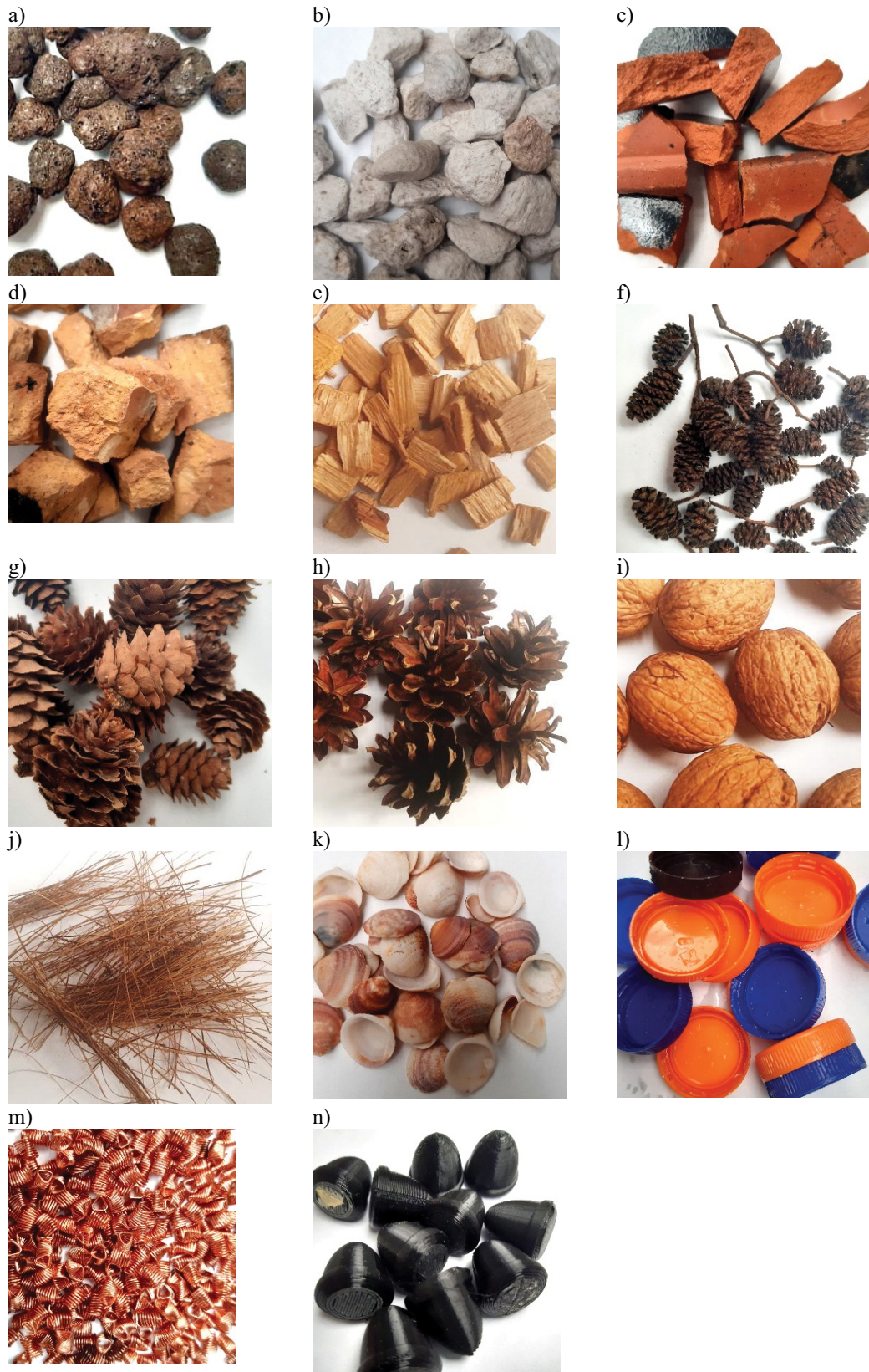
Fig. 1. Used packings: (a) LECA, (b) garden pumice of 10–20 mm, (c) Piedmont ceramic tile from Roben Company, (d) clinker brick, (e) wood chips, (f) black alder cones, (g) larch cones, (h) pine cones, (i) walnuts, (j) coconut fiber, (k) shells, (l) bottle caps, (m) prismatic springs, and (n) ABS acorns.
