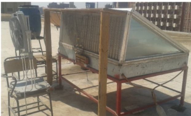
Fig. 9. Solar still with a heat sink integrated with a solar collector and a condenser and fan with an air-cooling flow [45] (Reprinted with permission from Elsevier).
