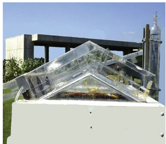
Fig. 17. A double-glass desalination unit with wind tunnel [67] (Reprinted with permission from Elsevier).
