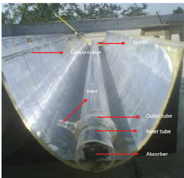
Fig. 16. Pictorial view of tubular solar still [62] (Reprinted with permission from Elsevier).
