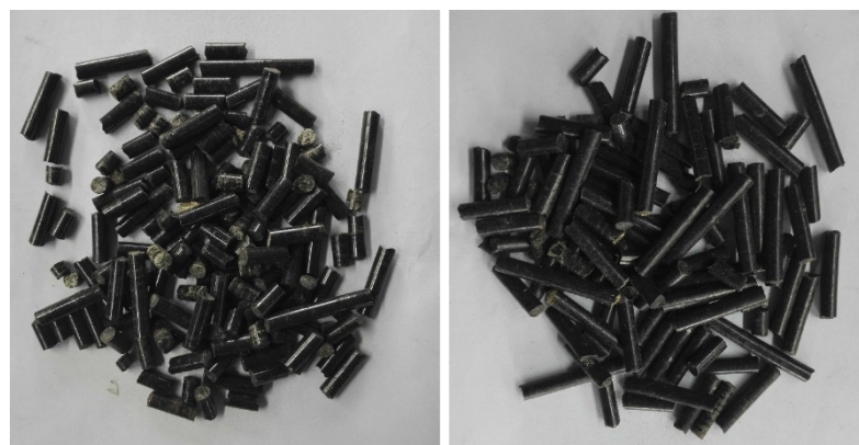
Fig. 3. Selected pellets of feedstock SS with organic additive and catalyst FS1.4 and FS2.2 (a) Mix4 feedstock of WWTP1 with wooden sawdust and (b) Mix1 feedstock of WWTP2 with crushed limestone, after pelletization process.
