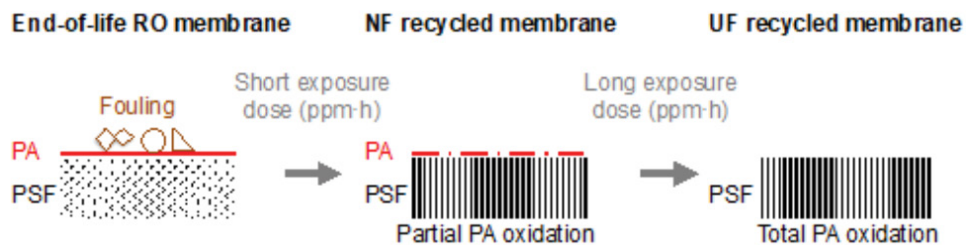
Fig. 1. Oxidation process of reverse osmosis membranes in nanofiltration or ultrafiltration membranes [26].
