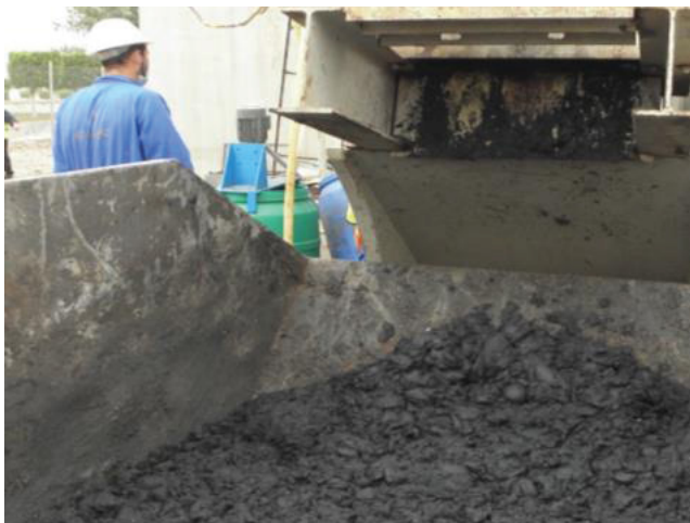
Fig. 2. Sludge cake delivered from the screw press machine.
