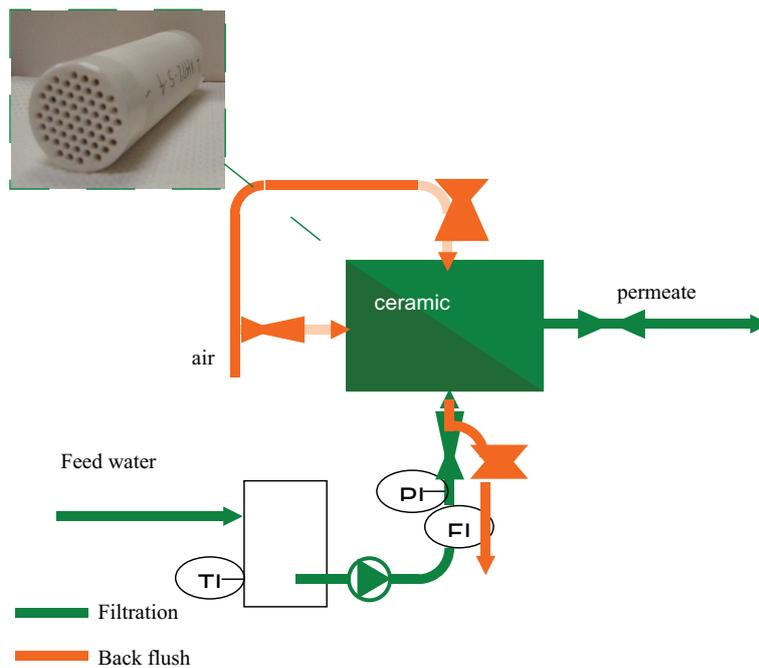
Fig. 4. Flow-sheet of the microfiltration unit.
