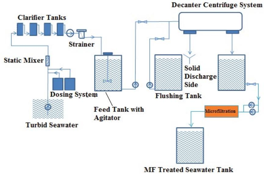
Fig. 2. Flow diagram of the decanter centrifugation unit.
