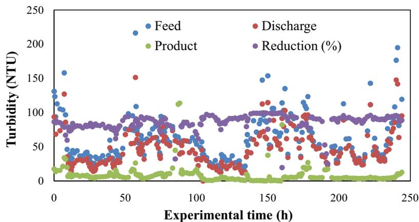
Fig. 9. Variation in feed, product, and discharge seawater turbidities during the decanter centrifugation treatment (50% closed mode) and percentage of reduction in turbidity after treatment.
