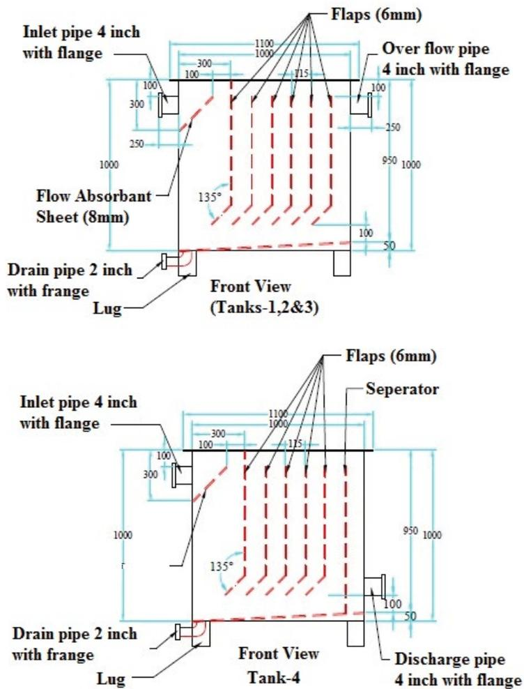
Fig. 3. Front view of the clarifier tanks.
