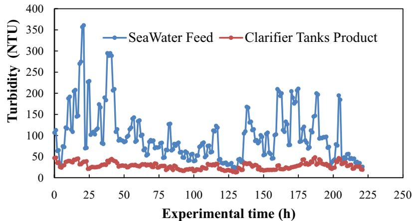
Fig. 8. Turbidities of seawater feed and clarifier tanks product vs. the number of readings.
