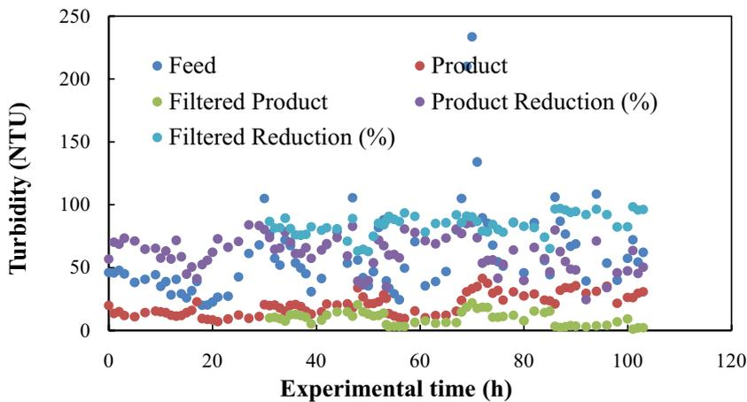
Fig. 7. Variation in seawater turbidity following the introduction of the filter after the decanter centrifuge system (fully open mode) and percentage of reduction in turbidity after treatment.
