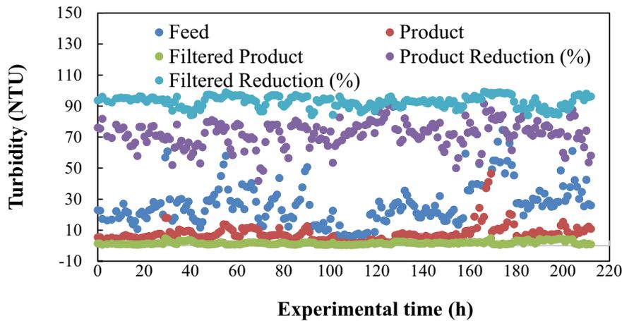
Fig. 10. Variations in seawater turbidity following the introduction of the filter after the decanter centrifuge system (50% closed mode) and percentage of reduction in turbidity after treatment.
