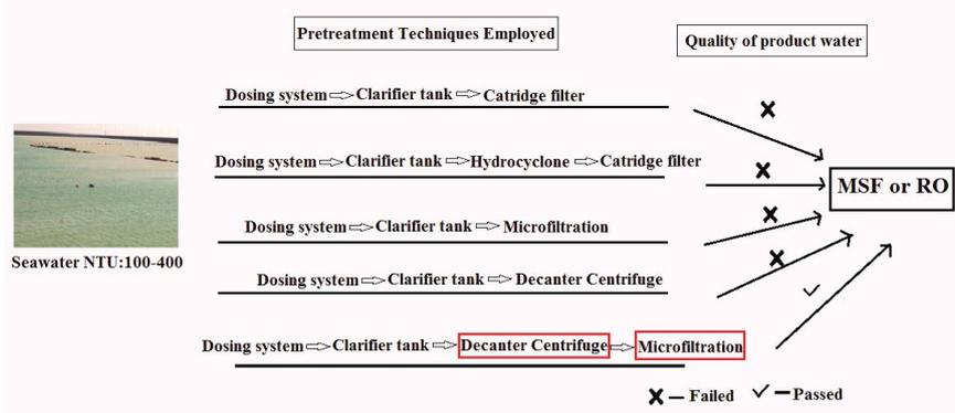
Fig. 12. Schematic presentation highlighting the success of the dosing system-clarifier tank-decanter centrifuge–microfiltration integrated system in providing the desired quality of feed water for both MSF/RO plants compared to other techniques adopted in the study
