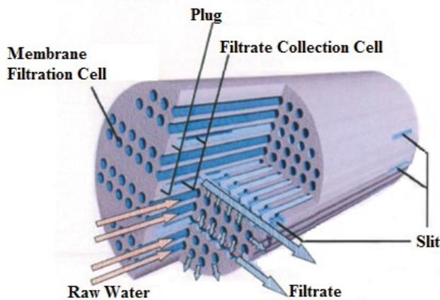
Fig. 5. Cross-sectional view of the ceramic membrane element.
