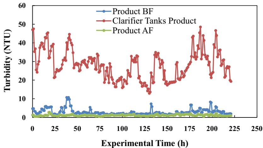
Fig. 11. Variations in seawater turbidity following the introduction of microfiltration after the decanter centrifuge system (before and after the MF treatment).
