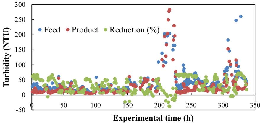
Fig. 6. Variation in feed and product seawater turbidities during the decanter centrifugation treatment (fully open mode) and percentage of reduction in turbidity after treatment.
