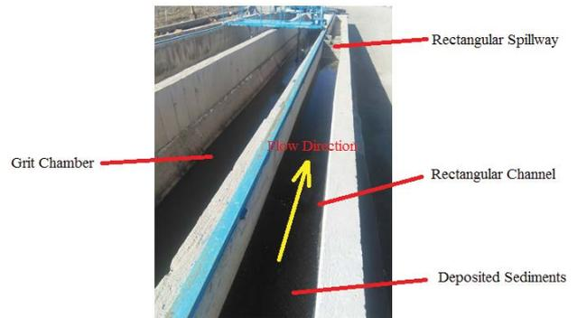
Fig. 1. Experimental setup of the rectangular concrete channel (upstream view).
