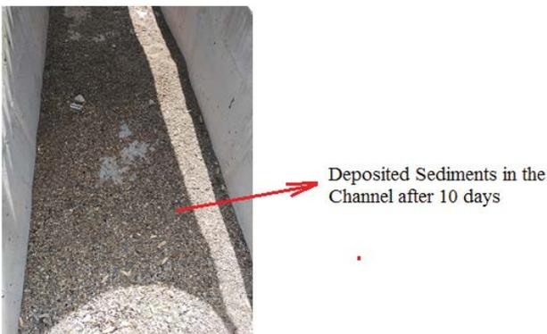
Fig. 7. Deposited sediments in the channel after 10 d to determine the gradation curve.
