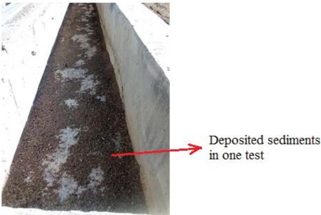
Fig. 6. Deposited sediments in the channel in one test to determine the weight of deposition.
