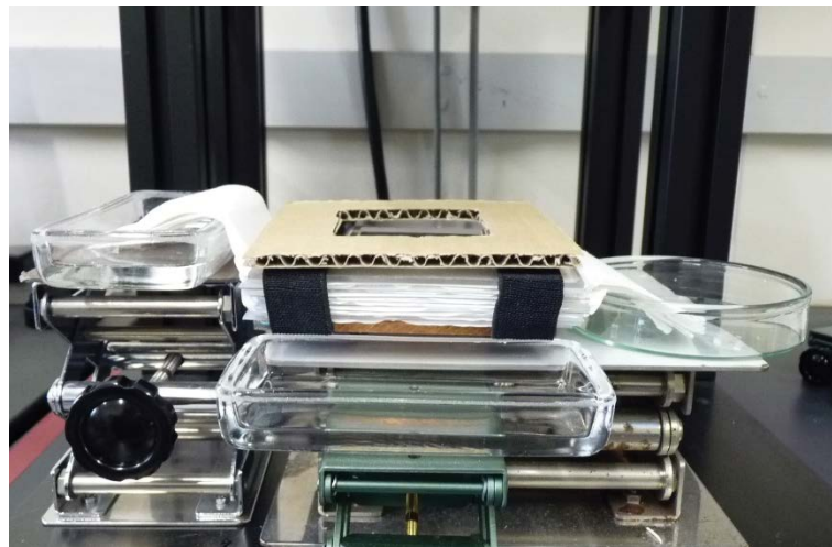
Fig. 4. An image of a ten-stage apparatus with water feeding by siphon mechanism.
