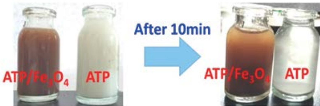
Fig. 7. Deposition of adsorbents in oil-water emulsion.
