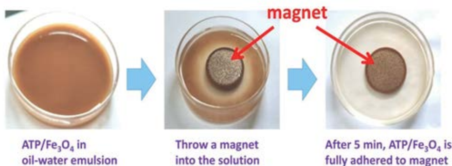
Fig. 8. Recovery efficiency of magnetic ATP from oil-water solution by strong magnetic field.
