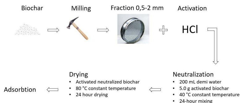
Fig. 1. Schema of preparing activated biochar.
