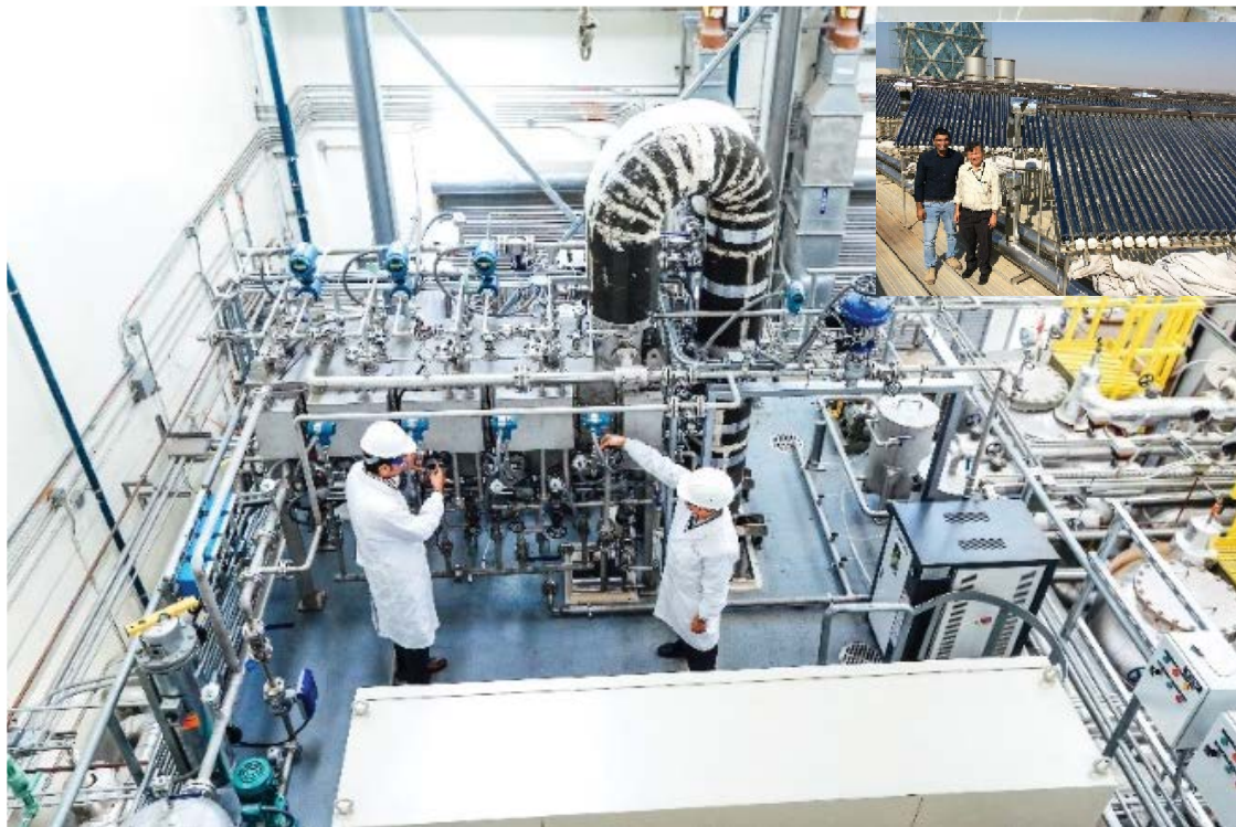
Fig. 5. Solar operated hybrid MED+PSAD pilot at KAUST, Saudi Arabia.
