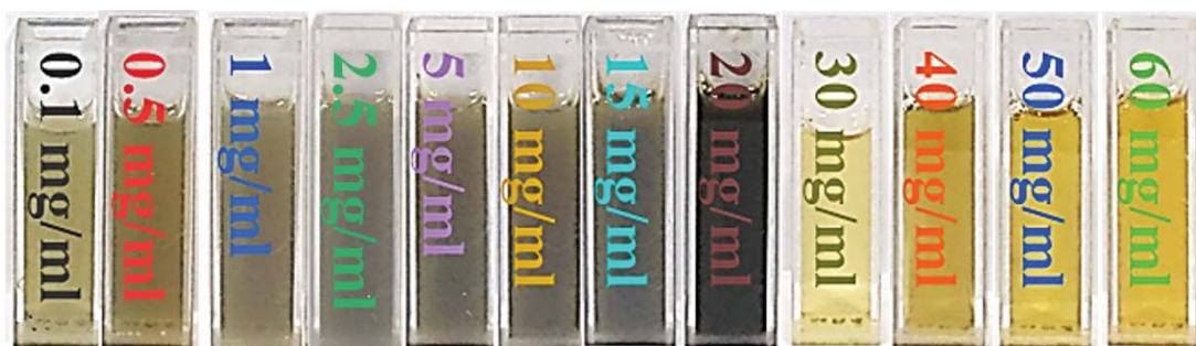
Fig. S3. Optical images of the dispersions of WS 2 nanosheets exfoliated at different chitosan concentrations for 10 h sonication.
