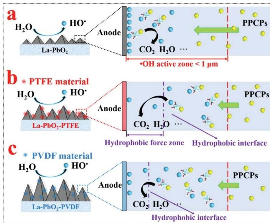
Fig. 2. Schematic diagram of degradation mechanism of PPCPs on the electrodes (Reprinted from Qian et al. [52], License Number: 5437510978948).
