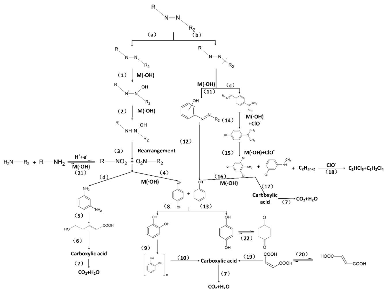
Fig. 3. General degradation process of azo compounds (R and R' represent different aromatic groups, respectively) [81,82,84–87].
