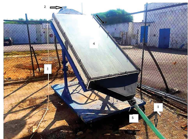
Fig. 1. Image of the solar evaporator: 1-air inlet, 2-humid air outlet, 3-water supply, 4-glass, 5-brine recovery.
