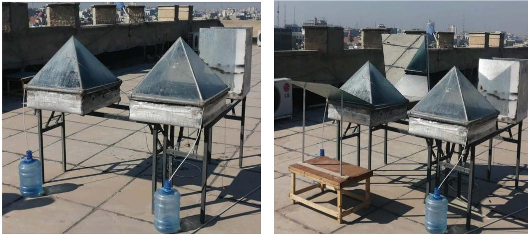
Fig. 1. Solar stills system (a) without reflectors and (b) with reflectors.
