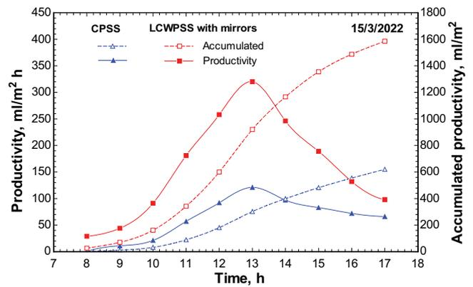
Fig. 7. The hourly variation in productivity and total accumulated productivity of both solar stills, CPSS and LCWPSS with reflectors.
