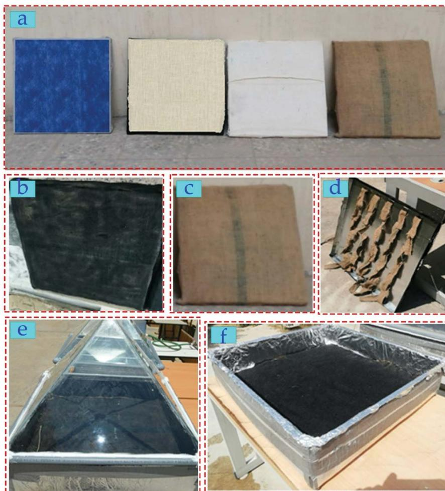
Fig. 3. Different arrangements of wick materials and cords (a) wick materials before the painting process, (b) black-painted jute wick, (c) jute wick, (d) back of jute wick, (e) wick inside SS, and (f) jute wick inside basin.
