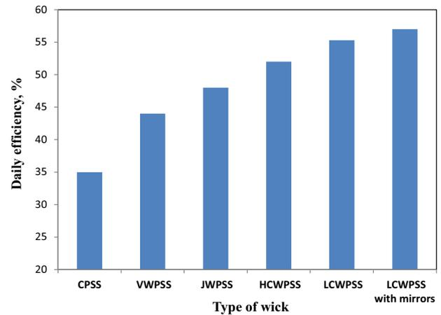
Fig. 8. Efficiency of CPSS and WPSS with different wick materials.
