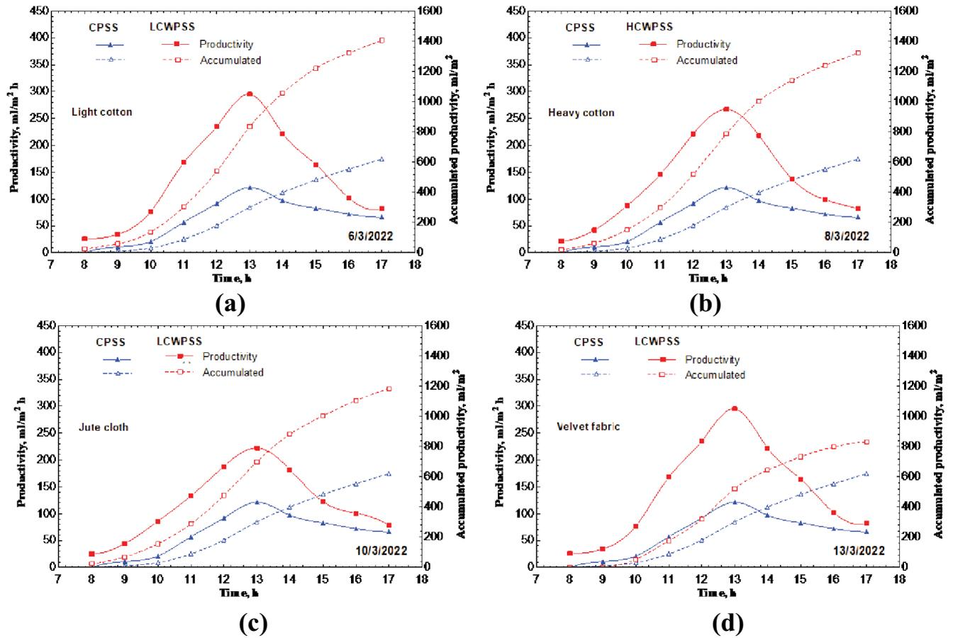
Fig. 5. Productivity hourly variation and overall cumulative productivity using different wicks, (a) light cotton, (b) heavy cotton, (c) jute fabric, and (d) velvet fabric.
