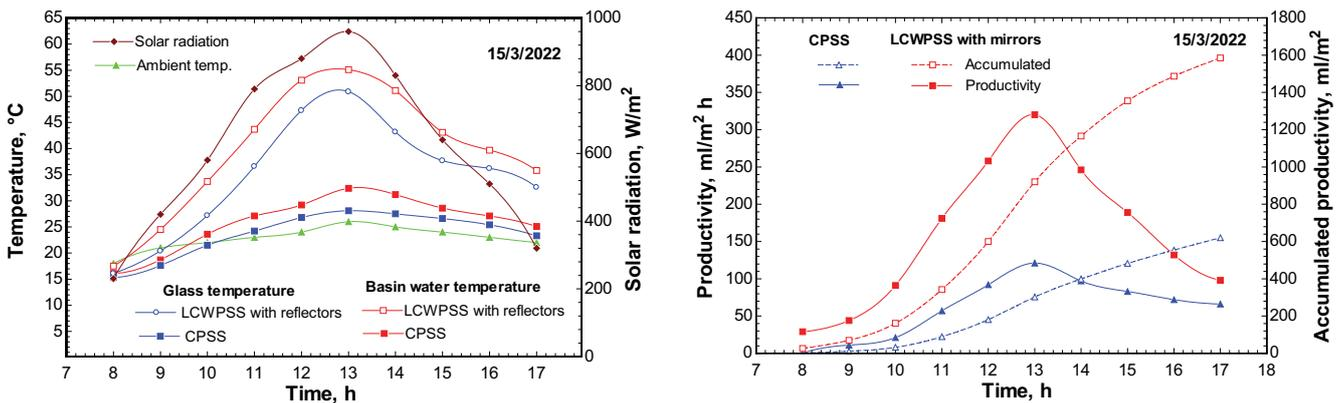
Fig. 6. Solar irradiation and temperature variations for the CPSS and LCWPSS with reflectors.
