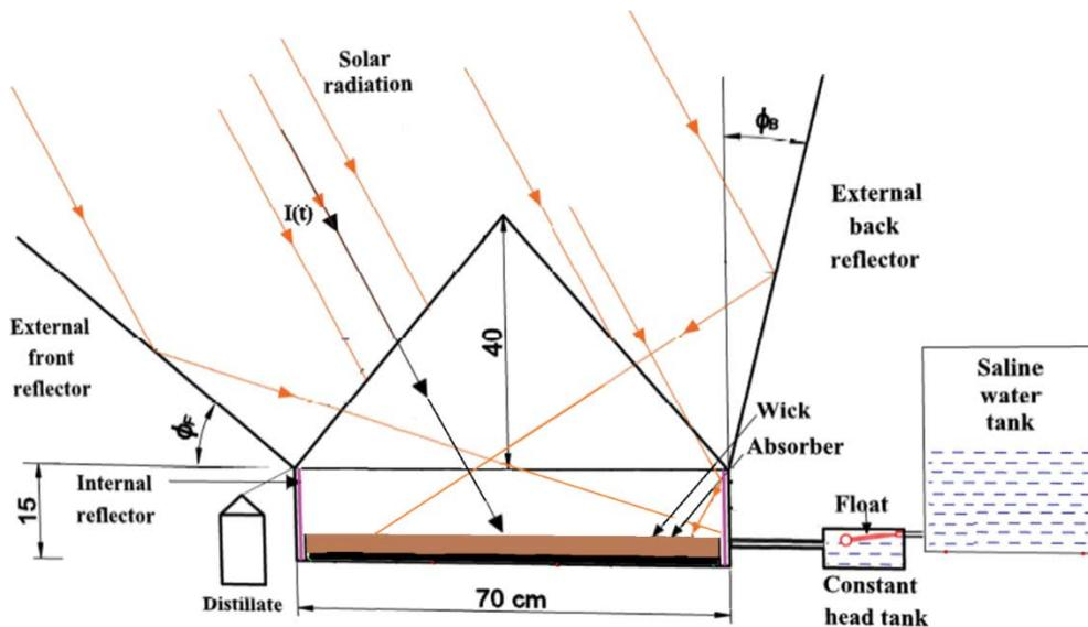
Fig. 2. Experimental test rig in two dimensions.
