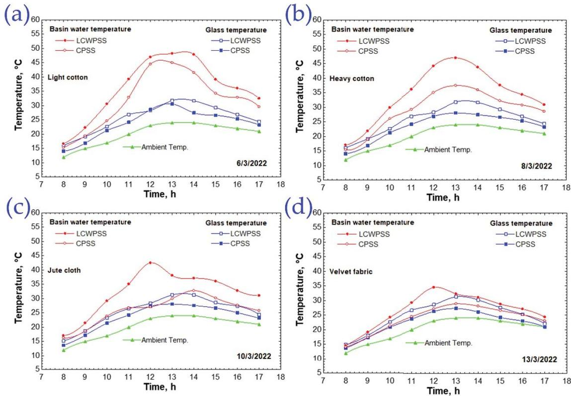
Fig. 4. Temperatures for the CPSS and WPSS with different wicks, (a) light cotton, (b) heavy cotton, (c) jute fabric, and (d) velvet fabric.
